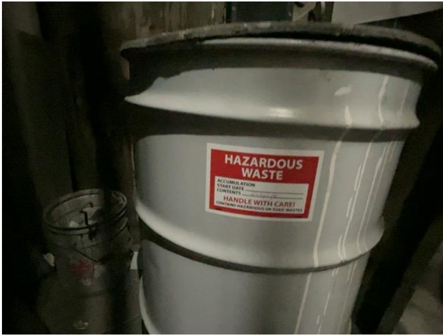
Photo 12 – Open SAA container in paint booth.
