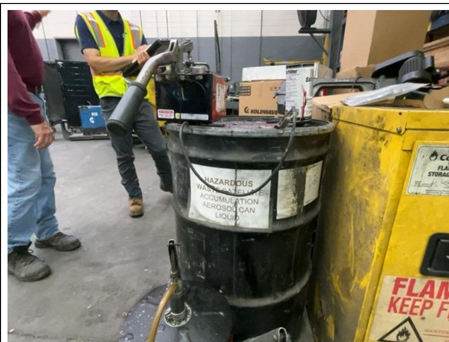
Photo 6 – Aerosol liquid SAA in the equipment maintenance area. This container was not marked with an indication of hazards of the contents.
