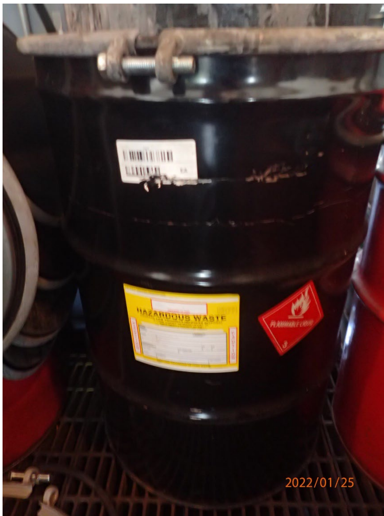
Photo 5: One (1) 55-gallon closed SAA drum of PPE and rags labeled “Hazardous Waste” and marked with an indication of hazard for flammability and toxicity.
