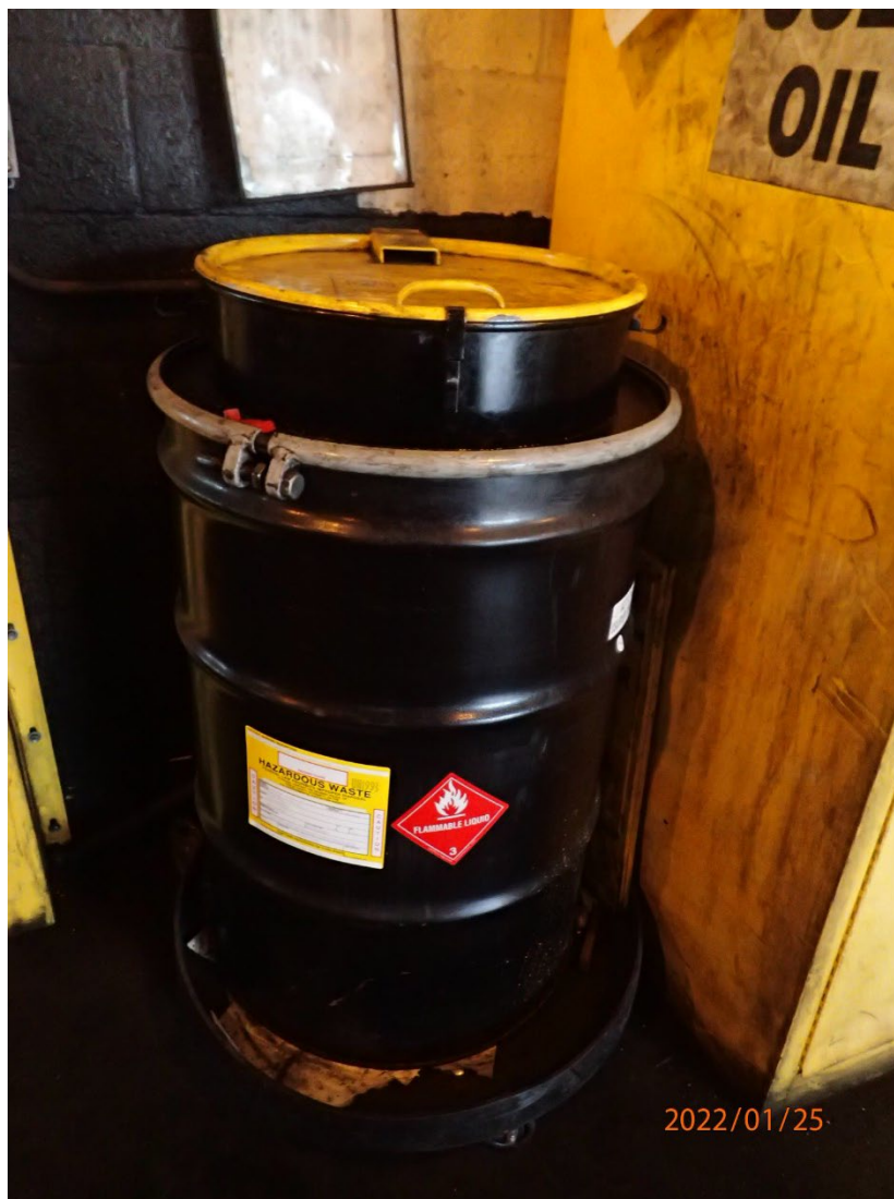
Photo 8: One (1) 55-gallon SAA closed drum of used oil samples from purges of material, labeled “Hazardous Waste”, and marked with an indication of hazard.
