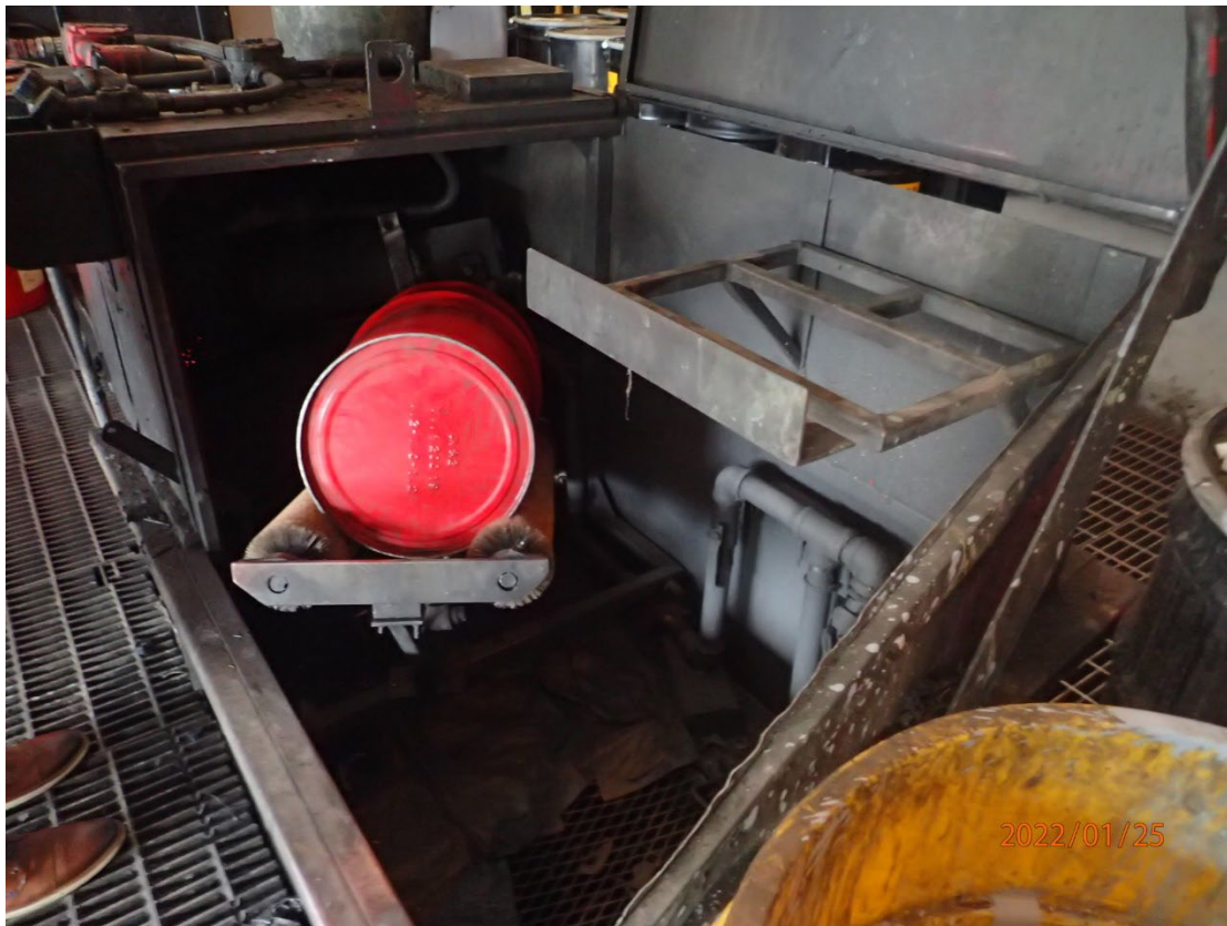
Photo 6: One red 55-gallon drum and spent solvent stored in one of the wet dumpsters.
