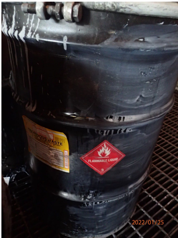
Photo 4: One (1) 55-gallon closed SAA drum of debris labeled “Hazardous Waste” and marked with an indication of hazard for flammability and toxicity.
