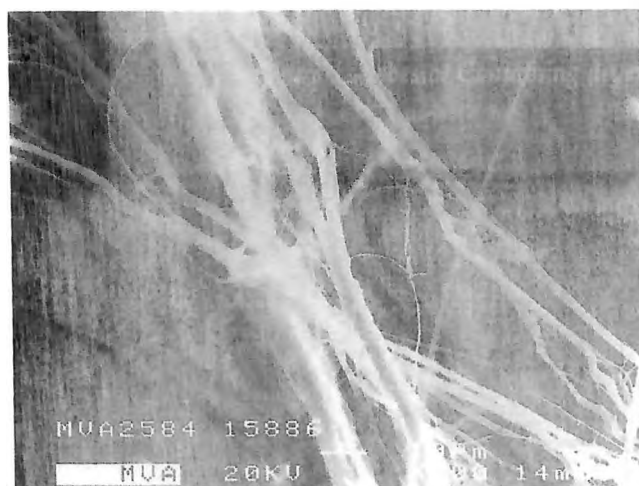
Figure 2. Scanning electron microscope image of chrysotile asbestos fibers released from the felt shown in Figure 1 onto a Post-it Note light adhesive sampler.
