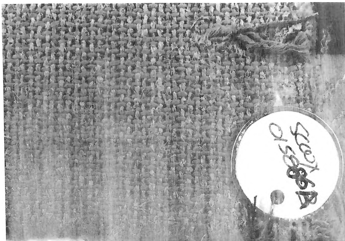
Figure 1. Asbestos Containing dryer felt textile, Sample 015886A as received.
