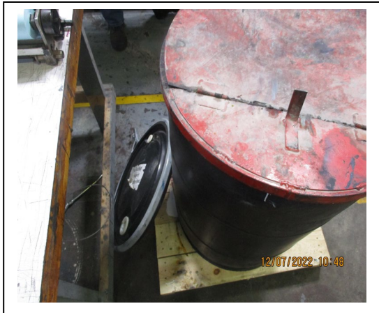
Photo # 5 – An open 55-gallon container of “Excluded Solvent Contaminated Wipes” with a lid on the floor.
