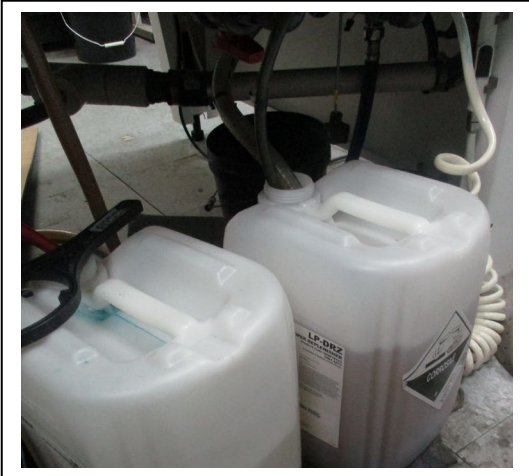
Photo #1 - open 55-gallon container of LP-DZ developer and LP-DRZ digital plate replenisher.
