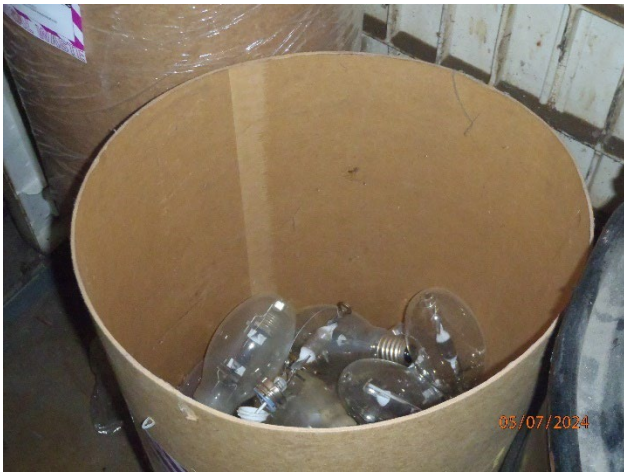
Picture 7 – Maintenance Universal Waste Storage open spent HID lamps
