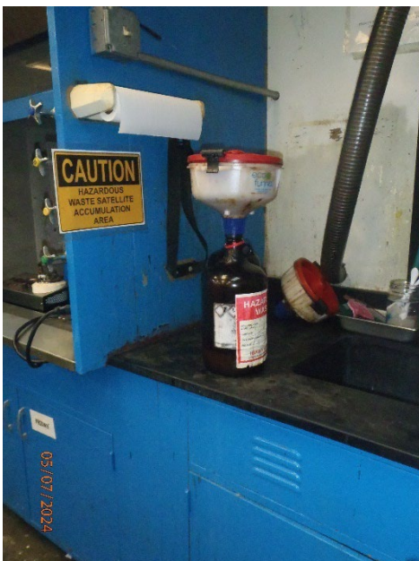
Picture 70 – Lab SAA containers
