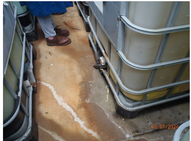
Picture 95 – Tanker Lot with clean out solvent tote leaking
