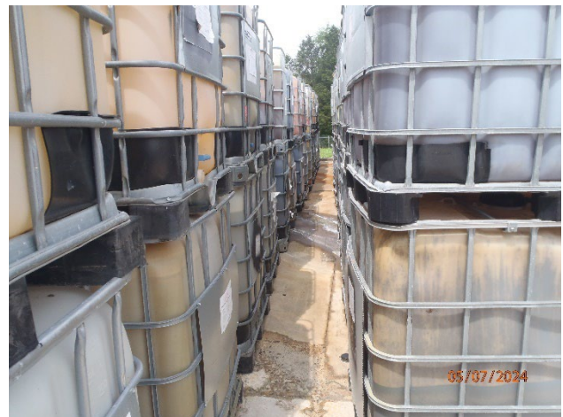
Picture 91 – Tanker Lot with clean out solvent release to ground
