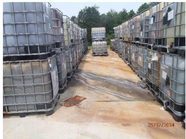
Picture 90 – Tanker Lot with clean out solvent release to ground
