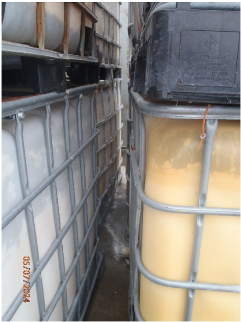
Picture 19 – Fatty Acid Tote Storage release to ground
