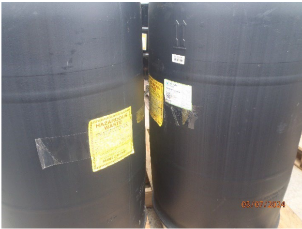
Picture 34 – HWCAA containers w/ damaged HW label
