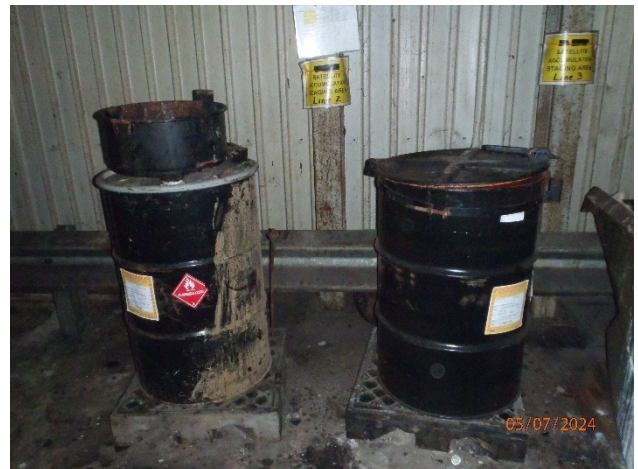
Picture 73 – Building 6 SAA open containers
