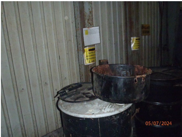
Picture 75 – Building 6 SAA open container
