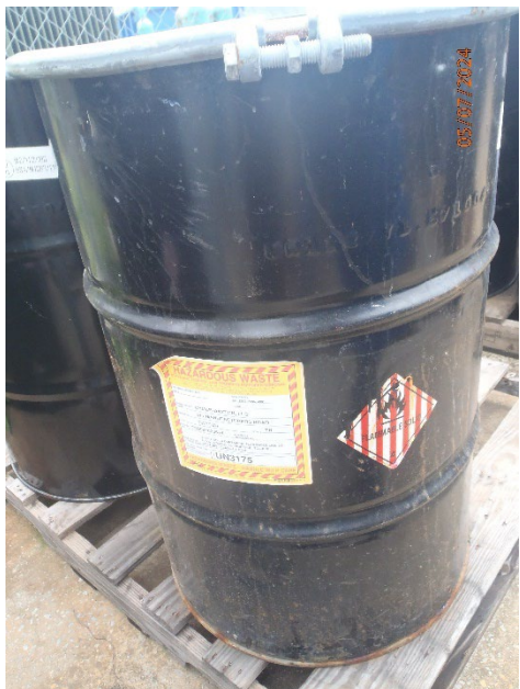
Picture 30 – HWCAA HW container missing date
