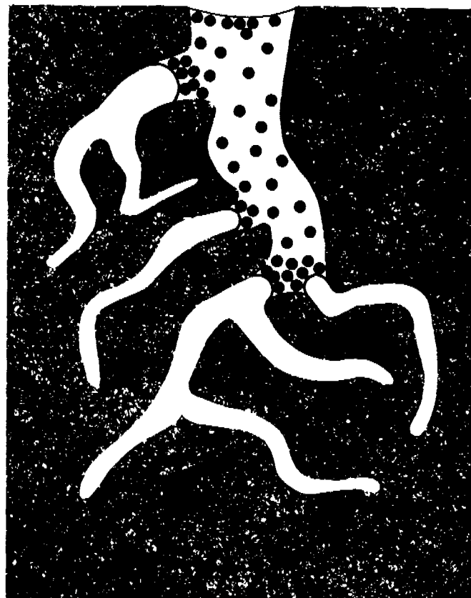
Figure 1b — Menisci formation by molecules in activated charcoal pores.
