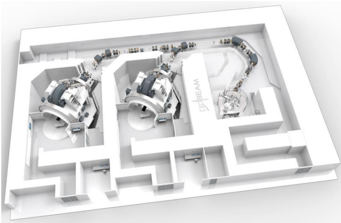
Figure 6: Schematic of a proton therapy centre
