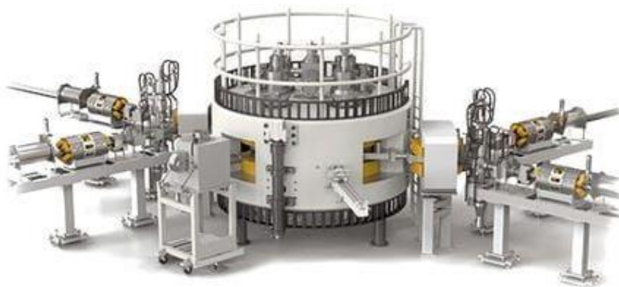
Figure 5: Cyclotron for proton beam generation in a Proton Therapy installation
