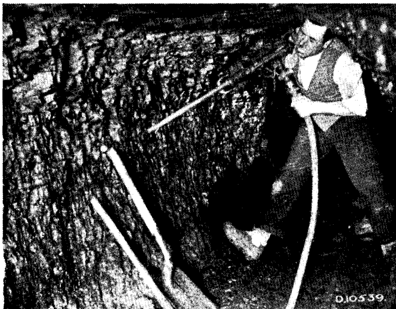
PLATE XX.—Drill of 1905 at work in narrow underhand stope (dry).
