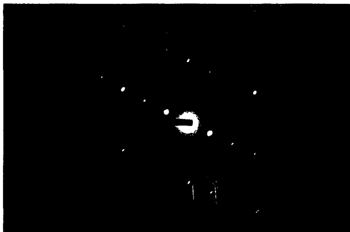
Figure 1b. SAED pattern of a talc ribbon with its (001) face oriented approximately parallel with the electron beam.
