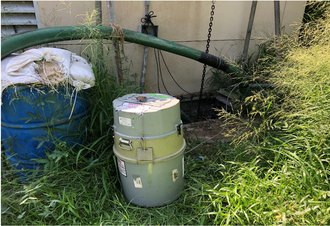
Photo #1. The automatic composite sampler was set-up at the influent wet well.
