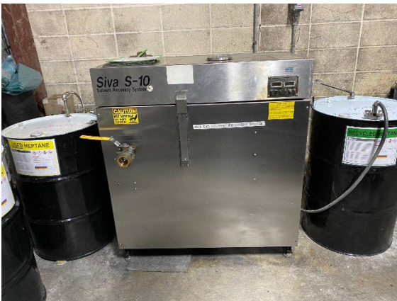
Photograph #11 – Siva S-10 solvent recovery system.
