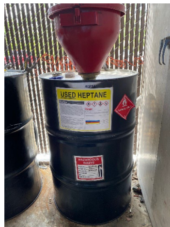
Photograph #6: 55-gallon container of used heptane without an indication of hazards “Toxic” label.
