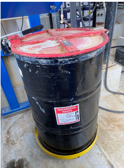
Photograph #9 – 55-gallon container of filter press sludge with no indication of hazards of the contents.
