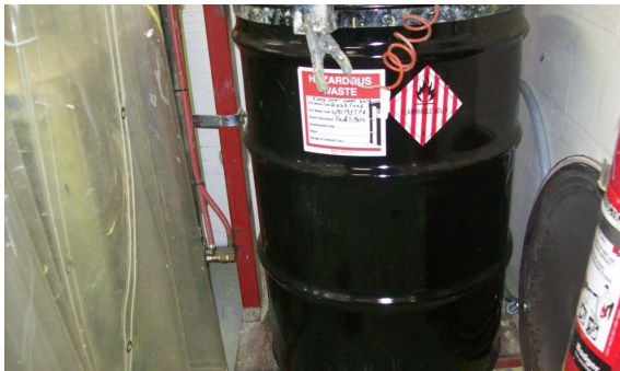
Photograph #3 – 55-gallon container of paint filter without an accumulation date.
