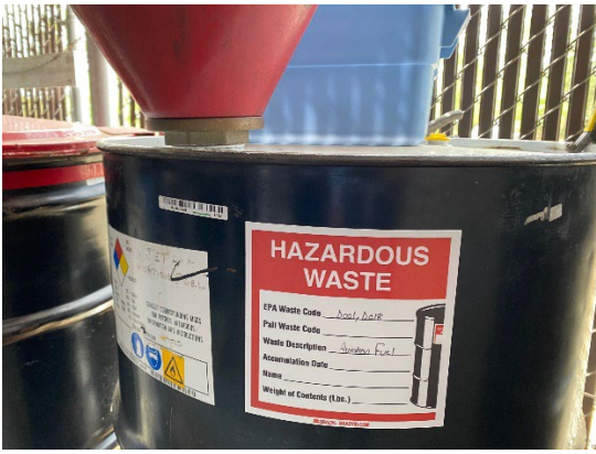
Photograph #7 – 55-gallon container of aviation fuel without hazards contents label.
