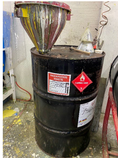
Photograph #4 - 55-gallon container of paint thinner without indication of hazards.
