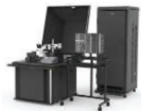
Static optical fault isolation for identifying process, design or integration issues
