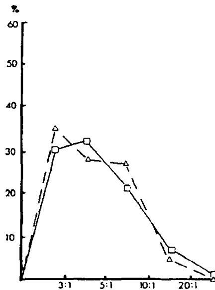
FIGURE 8. Percent amphiboles in each aspect group for a sample handled in two ways: solid line shows results using traditional method and dashed line shows results using centrifuge method. Dimensions of 100 particles measured for each curve.
