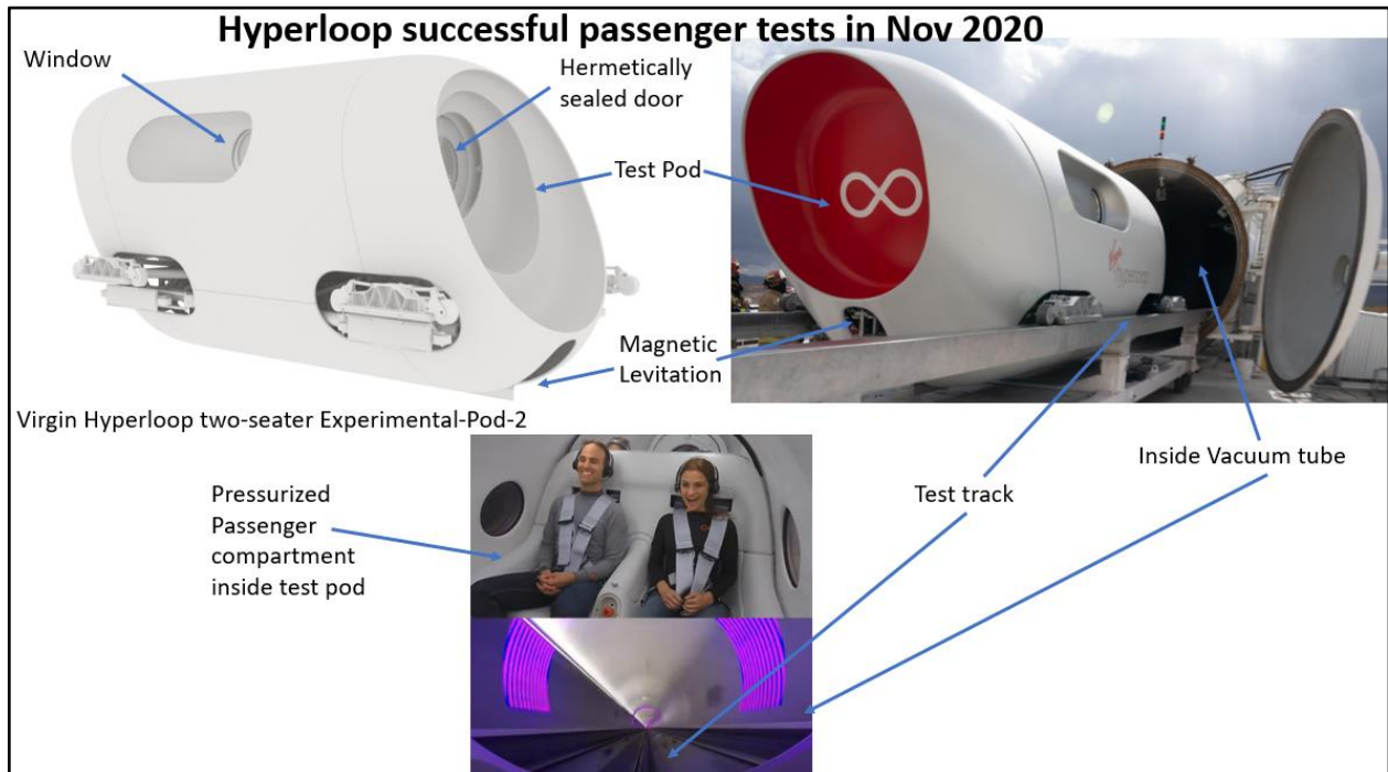
Figure 2: Hyperloop successful passenger tests conducted by Virgin Hyperloop in Nov 2020. Photographs source: Virgin Hyperloop (2020).
