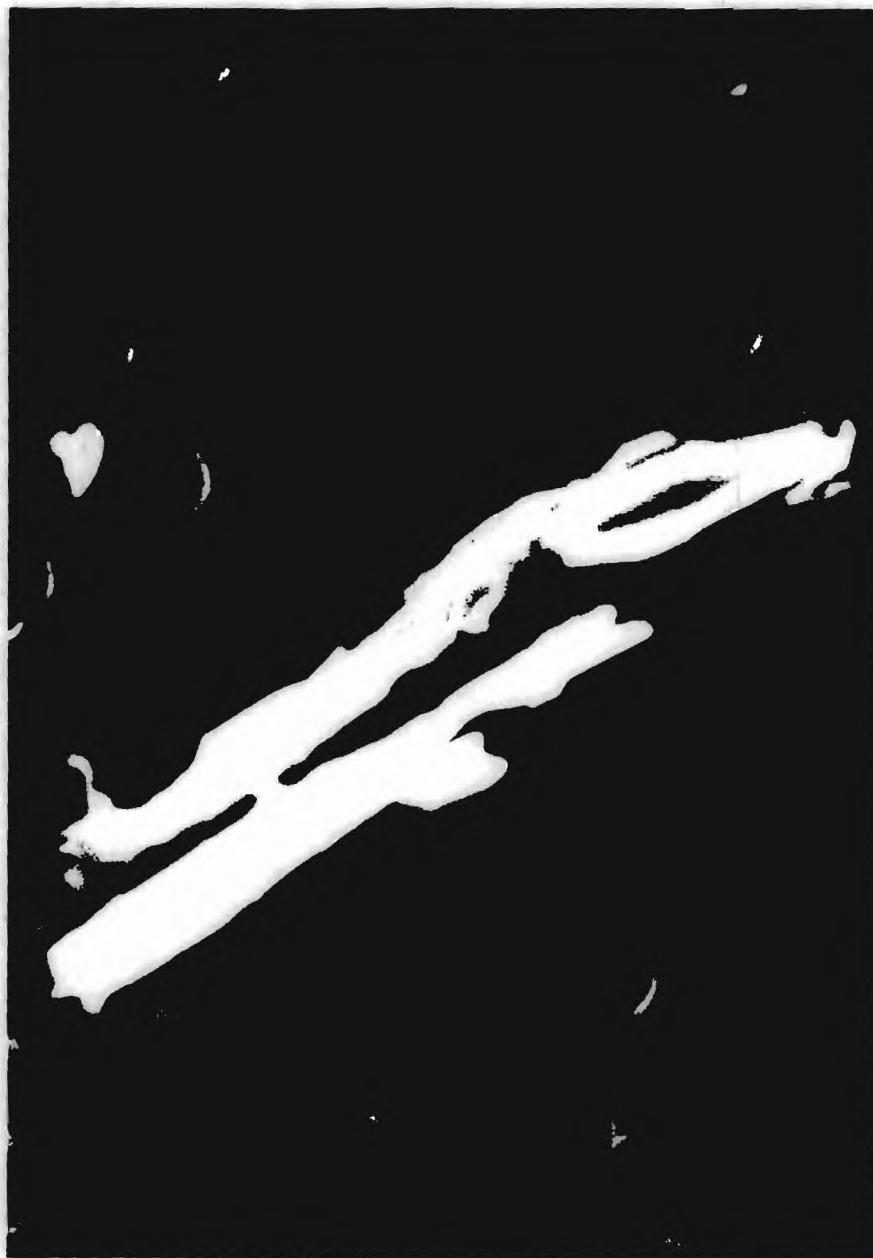
FIGURE 3. Scanning electron micrograph of one rolled talc particle at X12,000 which has curled on both sides to form a tube. At a lower magnification this particle would be counted as a fiber.
