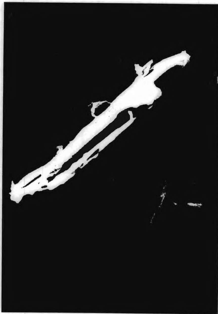
FIGURE 4. Scanning electron micrograph of an elongated particle standing on edge at X3500 magnification which might be considered as a fiber. By rotating the sample stage 60° (Figure 5), the laminated features of this talc particle can be seen.
