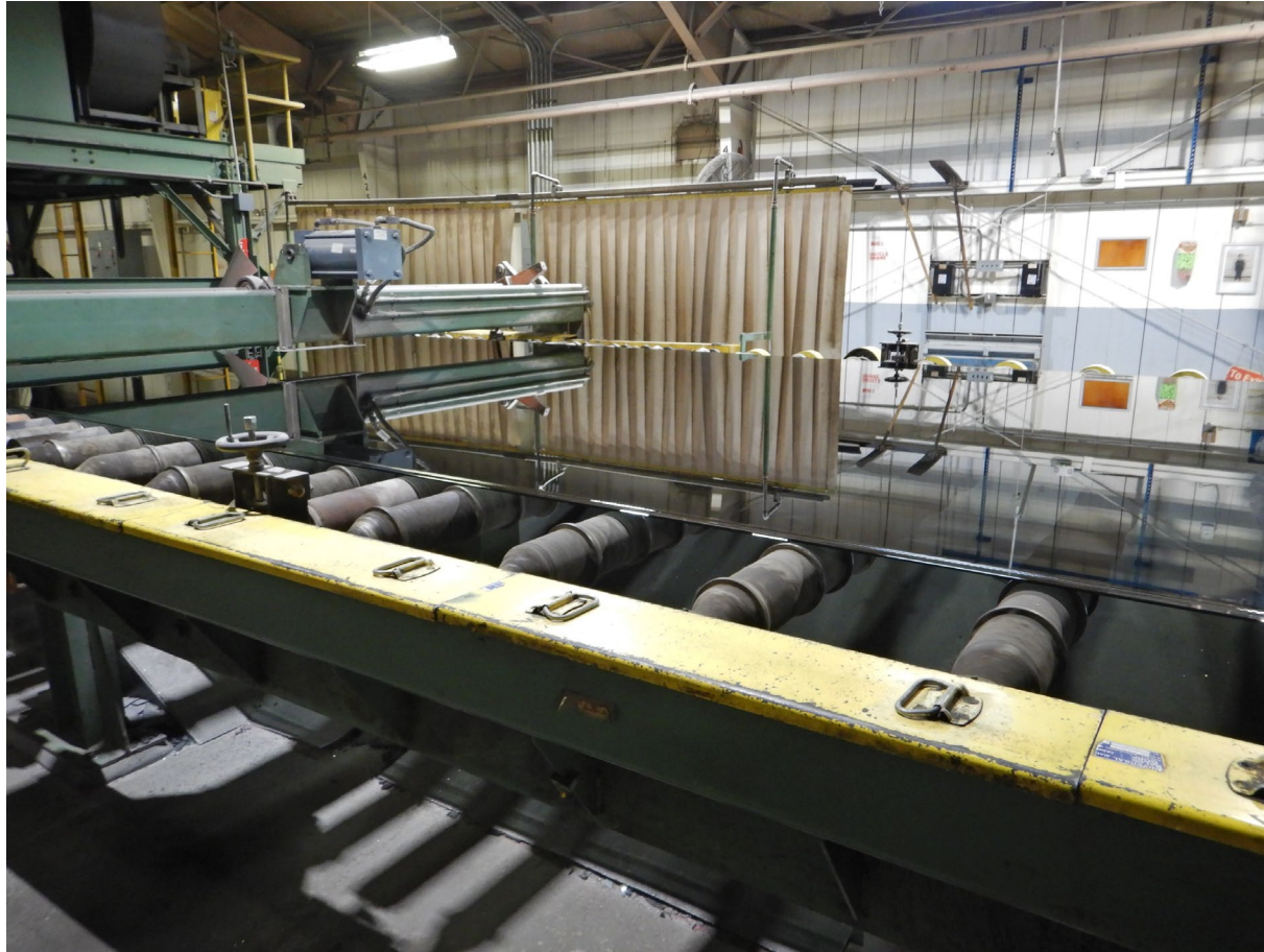
Photo 14 – Glass after annealing
