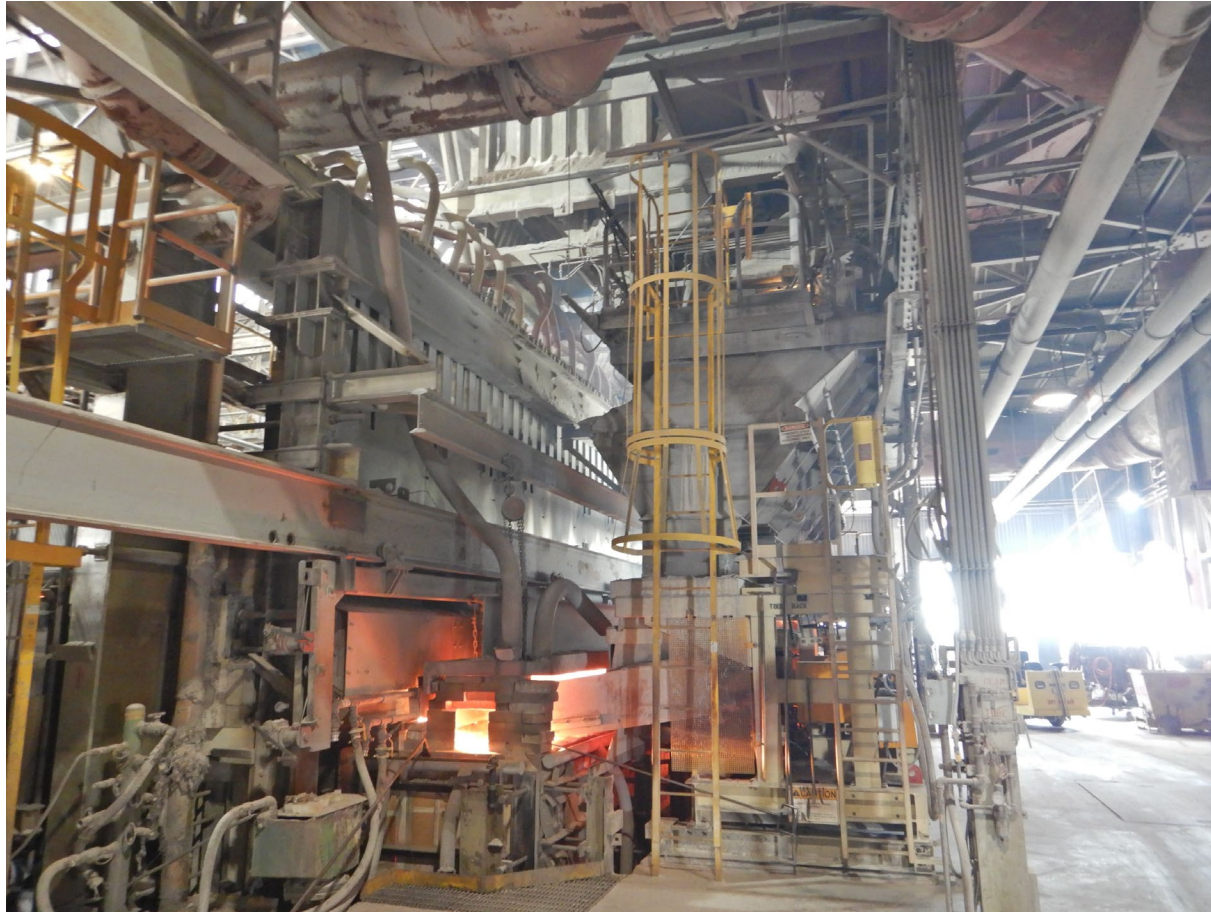
Photo 12 – Furnace hopper & pusher
