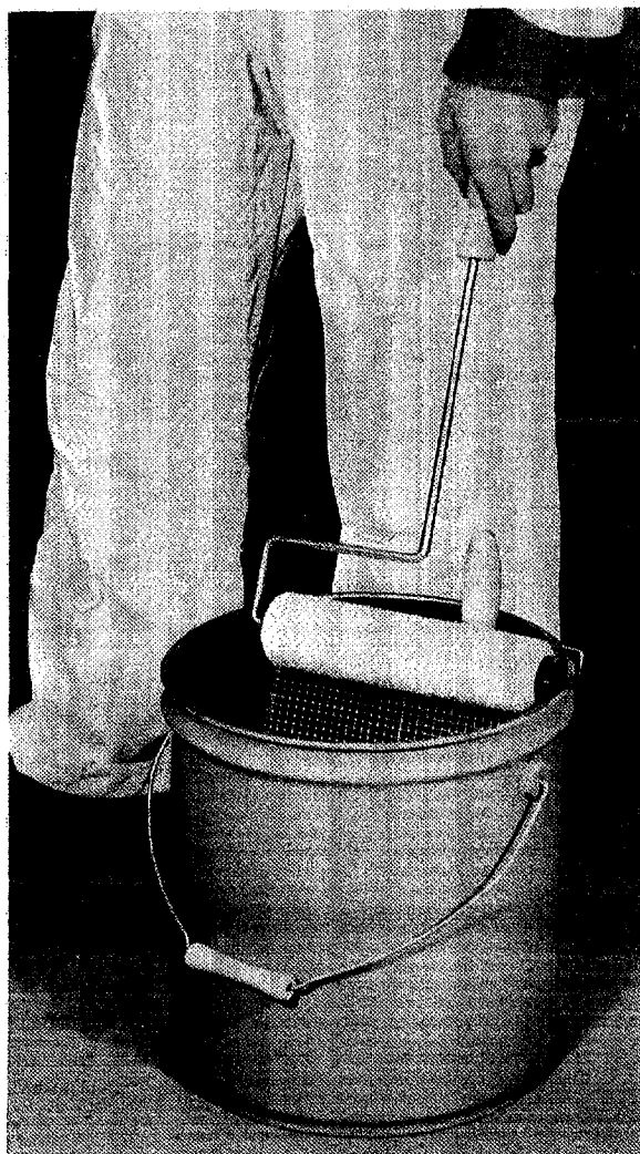
Figure 62. Roller and Wire Screen Attachment to Can.
