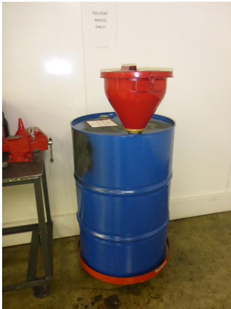
Photo 13: One 55-gallon container for accumulating purged liquid from restarting the doming process unit. The container is marked with waste profile number FC137581, labeled as non-hazardous waste, and identified with a flammable liquid hazard placard.
