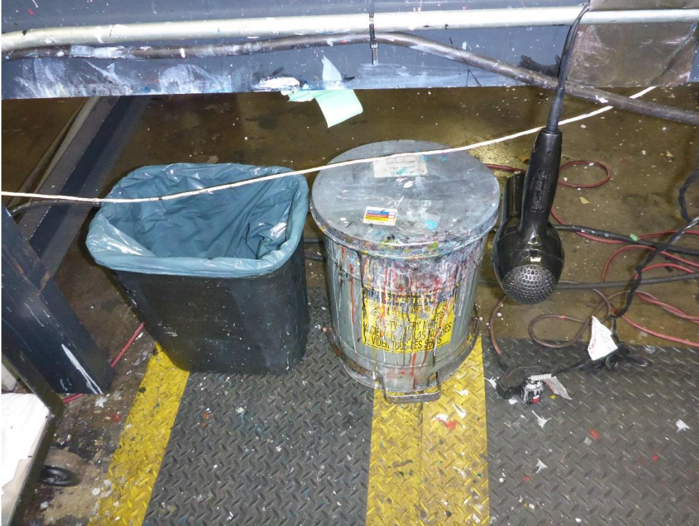
Photo 5: One flip-top 5-gallon container for accumulating solvent contaminated wipes in the Screen Print Area One. The container, which was located next to one of the screen print stations, was not labeled “excluded solvent contaminated wipes.”
