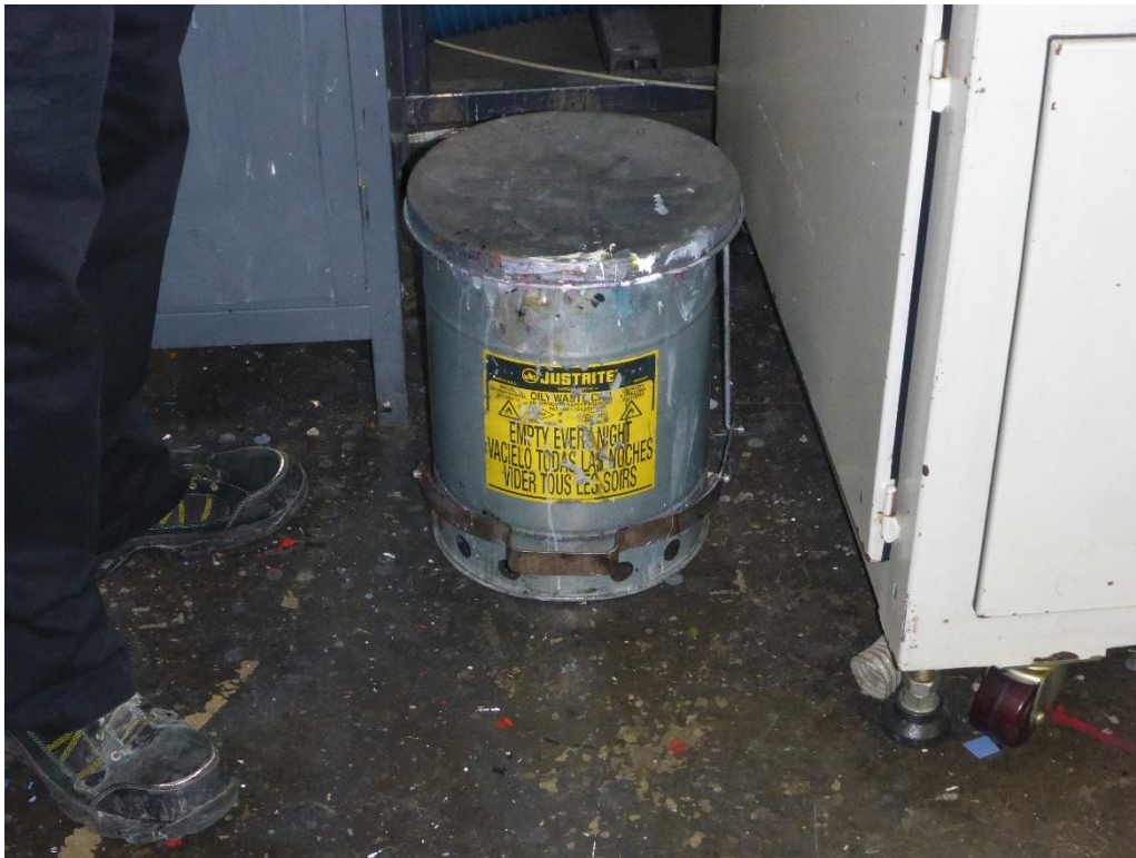
Photo 3: One flip-top 5-gallon container for accumulating solvent contaminated wipes in the Screen Print Area One. The container, which was located next to one of the screen print stations, was not labeled “excluded solvent contaminated wipes.”
