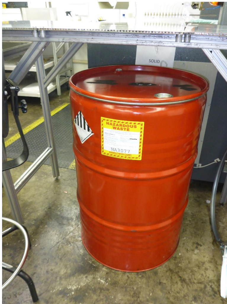
Photo 12: One 55-gallon container for accumulating D009 hazardous waste solid in the Doming Area. The container is labeled as D009 hazardous waste solid (mercury) and identified with a DOT class 9 hazard placard.
