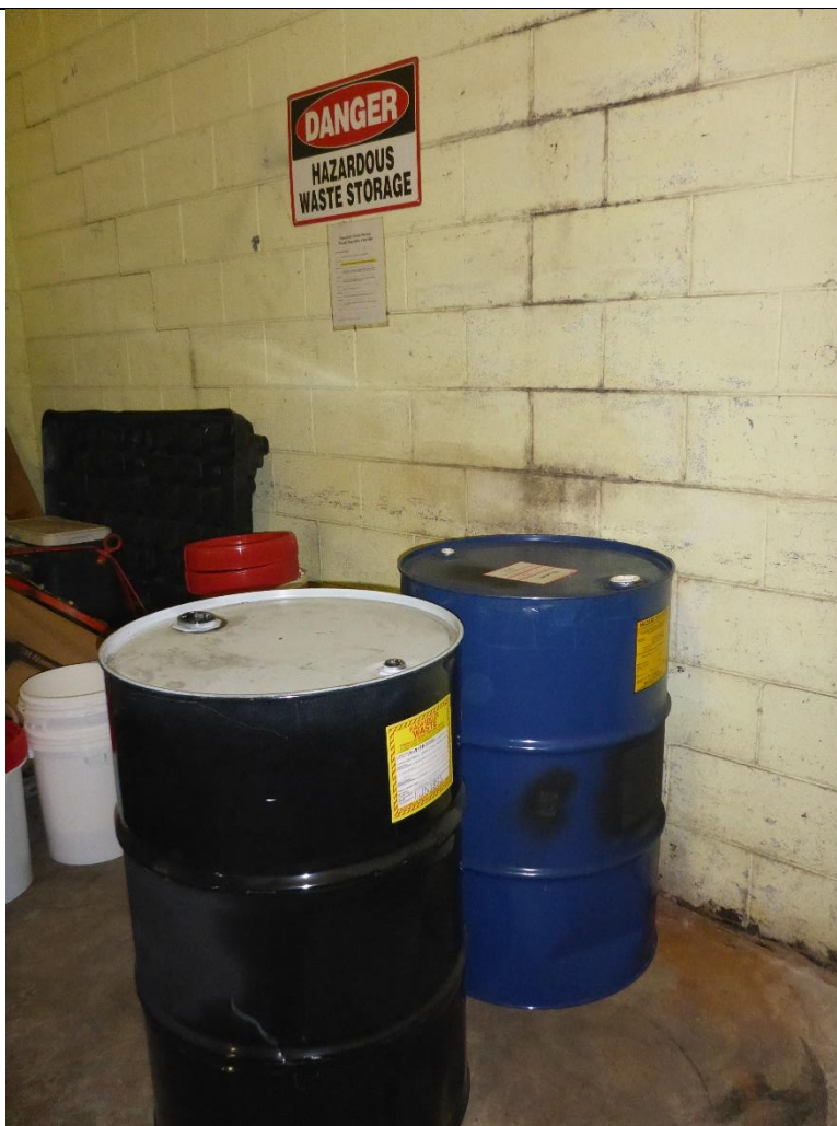
Photo 19: Two 55-gallon drums of hazardous waste in the Ink Shed CAA. The first drum was labeled as D001 / D035 / F005 hazardous waste flammable liquid (MEK) and identified with a flammable liquid hazard placard. The second drum was labeled F005 / F003 / D001 / D035 hazardous waste roll coat wash waste flammable liquid (MEK), and it was identified with a flammable liquid hazard placard. Both drums were closed and marked with an accumulation start date.
