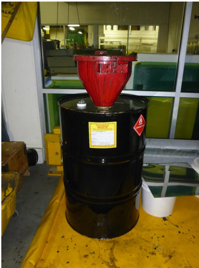
Photo 8: One 55-gallon container for accumulating hazardous waste generated in the Roll Coat Area Two. The container is labeled as D001 / D035 / F005 hazardous waste flammable liquid (MEK), and identified with a flammable liquid hazard placard. The small bung on the lid of the drum was open.
