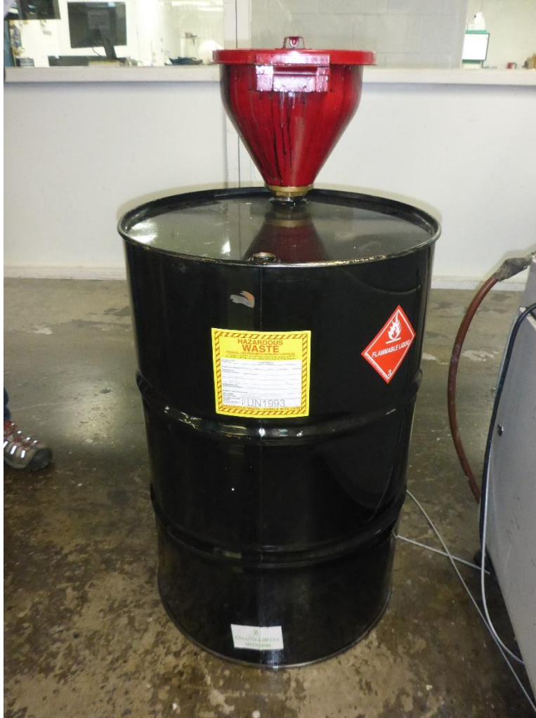
Photo 2: One 55-gallon container for accumulating hazardous waste generated in the Screen Print Area One. The container is labeled as D001 / D035 / F005 hazardous waste flammable liquid (MEK), and identified with a flammable liquid hazard placard.
