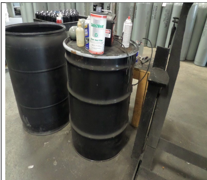
Chlorine Packaging. Inspectors observed a 55-gallon SAA container of spent solvent from aerosol puncturing. Observed not marked or labeled with the words hazardous waste and not marked or labeled with a hazard indicator. Brenntag representatives labeled the container. Photograph 9 taken at 11:37 a.m.
