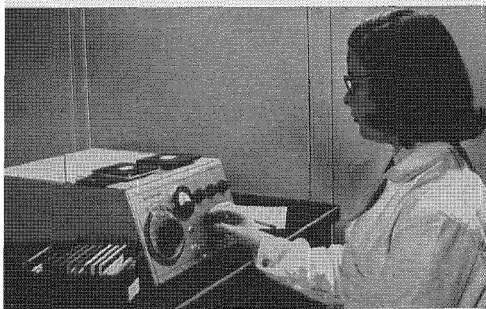
This colorimeter has helped reduce by half the shadings required to put a batch of finish within color specifications.
