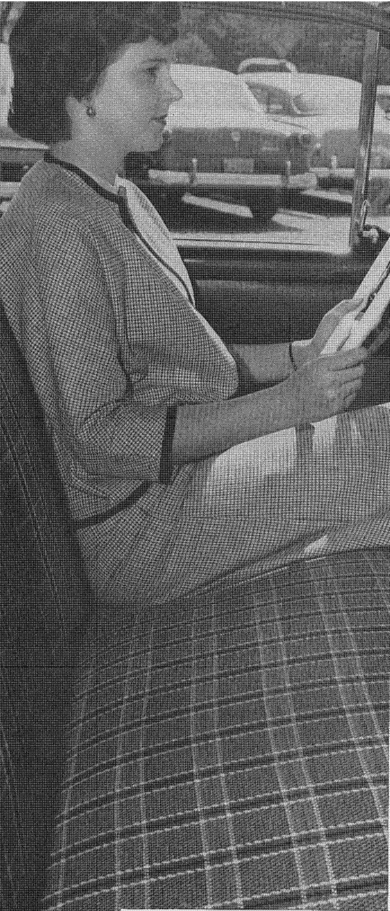
An example of the new water-resistant fiber seat covers made of neoprene-treated paper.
