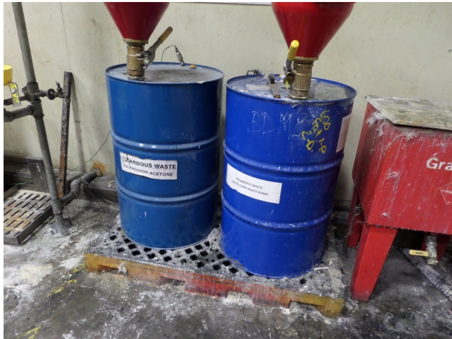
Photograph 6: Spent acetone from cleaning activities (D001/F003) and spent resin catalyst (D001) from the resin coating process generated in the Pultrusion Area. The containers were neither marked nor labeled with an indication of the hazards of their contents.
