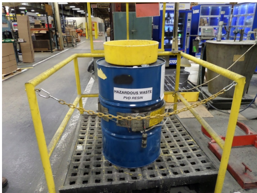
Photograph 2: “Hazardous Waste PVD Resin” 55-gallon container near the ARBU resin station, the inspectors observed a 55-gallon container labeled (Photograph 2). The container was being used for treatment of the activated resin.
