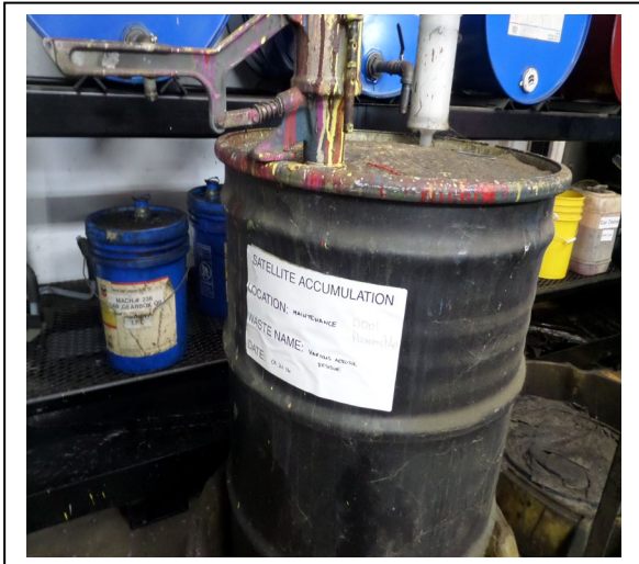
Hager. Maintenance Shop. Inspectors observed a 55-gallon SAA container not labeled/marked as hazardous waste and no hazard indicator. Photograph 3 taken at 10:24 a.m.
