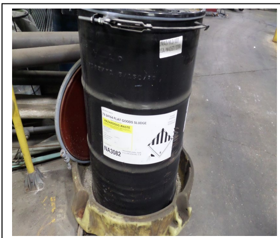
Hager. Oxidizing Line. Inspectors observed a DOT Class 9 (miscellaneous hazardous materials) pictogram on the 55-gallon SAA container. The inspectors observed the container appeared not labeled or marked with an indication of the hazard of the contents. Photograph 8 taken at 10:45 a.m.
