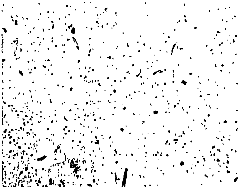
Figure 4. Even distribution of asbestos and non-asbestos particles as collected with the modified filter holder (1-3/4" long plenum) and viewed at 500X, phase contrast. (Sample D)
