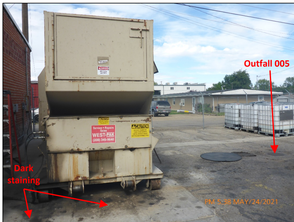
Photograph 39. View, facing east, of dark staining on the impervious surface underneath the trash compactor upgradient of Outfall 005, shown in Photographs 10, 33, and 38.
