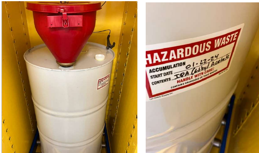
Photo #14 – Bldg. #3 Cleaning Room: One (55)-gallon container with IPA ethyl acetate waste
