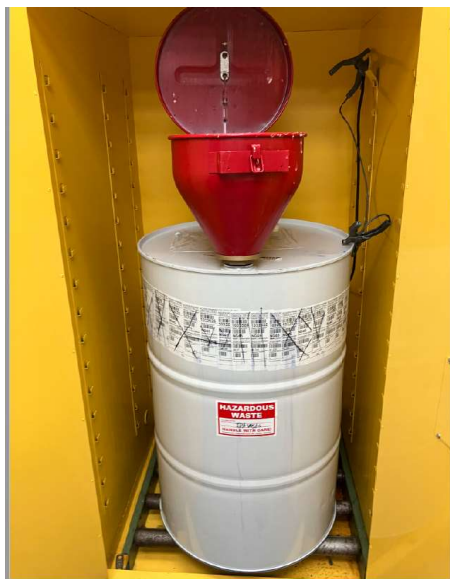
Photo #5 – Bldg #2: Cleaning Room: A (55)-gallon container with IPA waste, opened funnel. The container was not marked with the indication of the hazard of the content.
