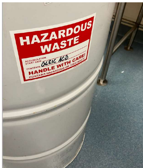
Photo #4 – Bldg #2: Cleaning Room: A (55)-gallon container. The container was not marked with the indication of the hazard of the content.
