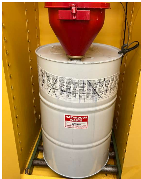
Photo #5 – Bldg #2: Cleaning Room: A (55)-gallon container with IPA waste, opened funnel. The container was not marked with the indication of the hazard of the content.
