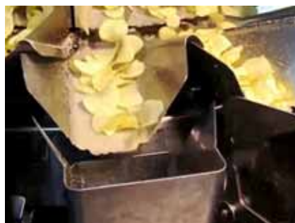
Example of oil accumulation (Food contact part is a flat stainless steel without coating)
