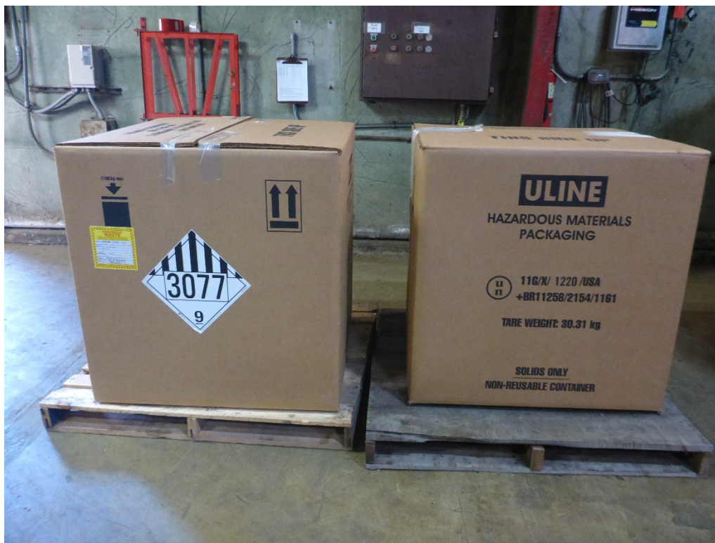
Photo 3: Two cubic yard boxes of used gloves, respirator cartridges and other PPE, empty product bags and contaminated trash in the CAA. Each box was labeled D007 / D008 hazardous waste solid and identified with a DOT class 9 hazard placard. One box was dated 11/16/2021 and the other was dated 09/21/2021.
