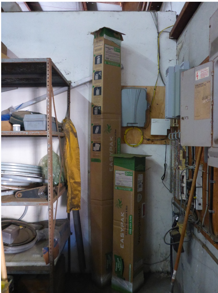
Photo 1: One box of 4-ft used fluorescent lamps and one box of 8-ft used fluorescent lamps in the Warehouse. Both boxes were closed and labeled as universal hazardous waste lamps. The 4-ft box was marked with an accumulation start date of 04/22/2021 and the 8-ft box was marked with an accumulation start date of 03/29/2021.
