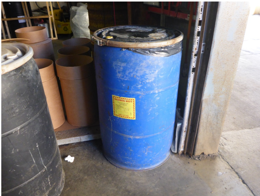
Photo 2: SAA One 55-gallon drum in the Warehouse SAA for managing empty raw material bags, used PPE and contaminated trash as hazardous waste solids. The drum was closed and labeled D007 / D008 hazardous waste solids, but it was not marked with an indication of the hazards of its contents.
