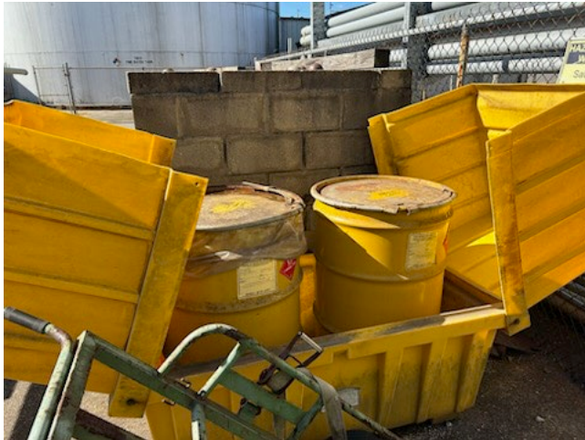
Photo 5: Two 55-gallon containers inside a clam-shell-type storage unit at the Maintenance Area SAA.
