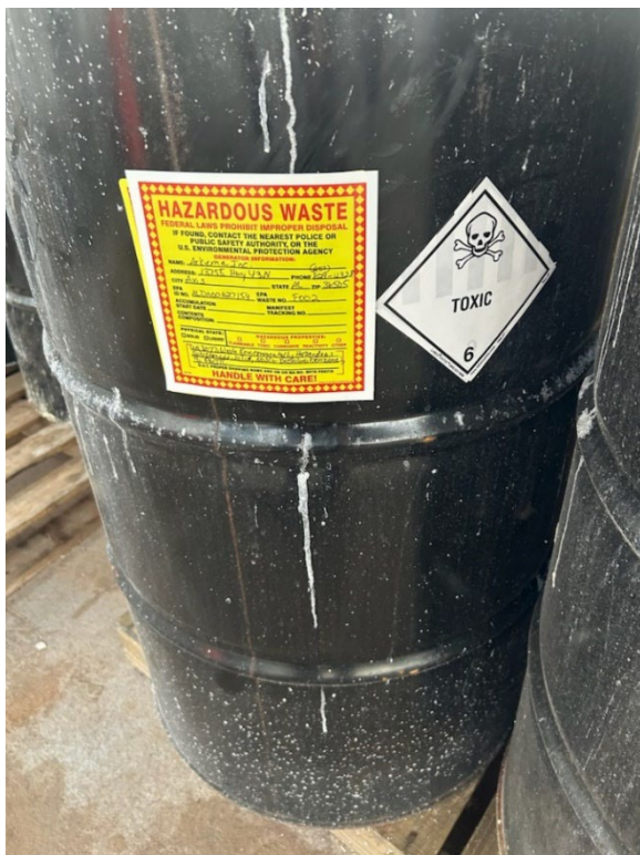
Photo B: Following the inspection tour of facility operations, a DOT toxic hazard sticker was added to the container of F002 hazardous waste environmental hazardous substance that was observed on Pallet 01 in the CAA.
