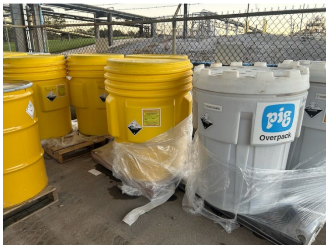
Photo C: Following the inspection tour of facility operations, DOT corrosive hazard stickers were added to overpack containers that were observed on Pallets 04, 05, and 06 in the CAA.
