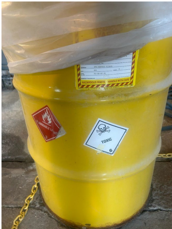
Photo H: Following the inspection tour of facility operations, a DOT toxic hazard sticker was added to the 55-gallon container in the Phase 0 PA Process Area SAA.
