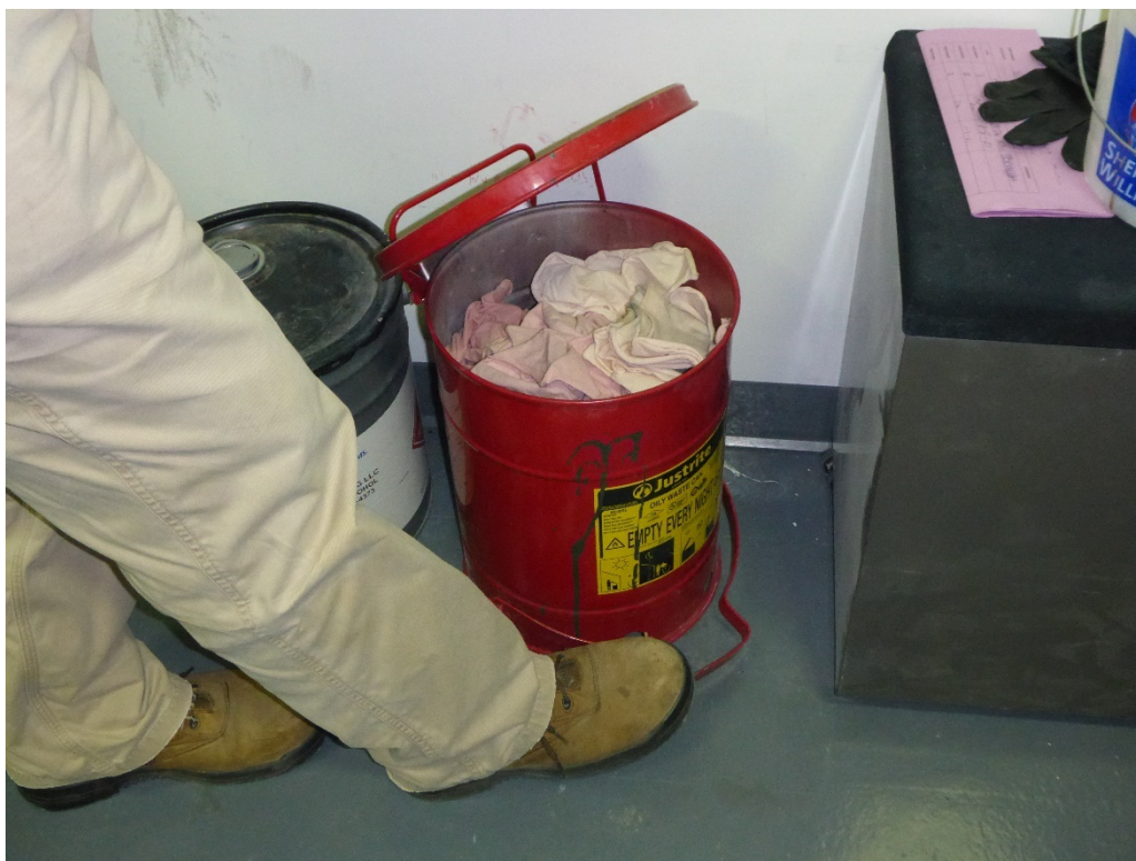
Photo 21: One 5-gallon step-open flammable can for accumulating excluded solvent contaminated disposable wipes at the laquer spray line. The container is labeled as “oily waste” and “empty every night.” It is not labeled as excluded solvent contaminated wipes.
