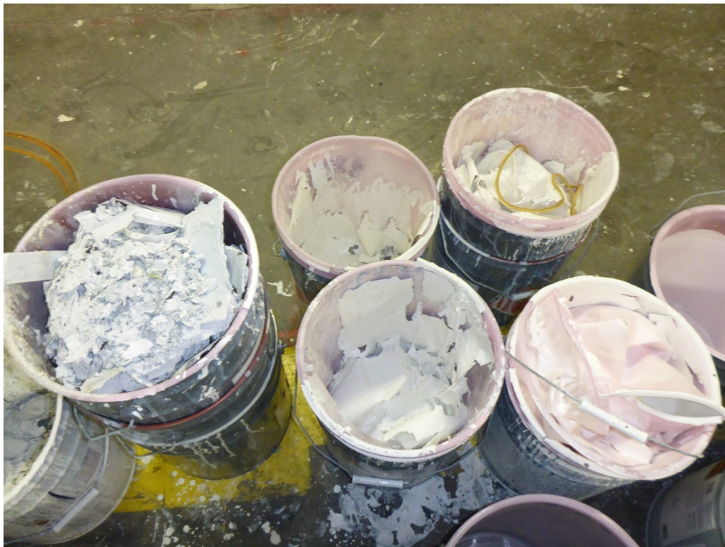
Photo 12: Several of the 5-gallon buckets with and without liners in the Reclaim Room. Buckets and liners appear to contain UV paint waste. The buckets are open and not labeled.
