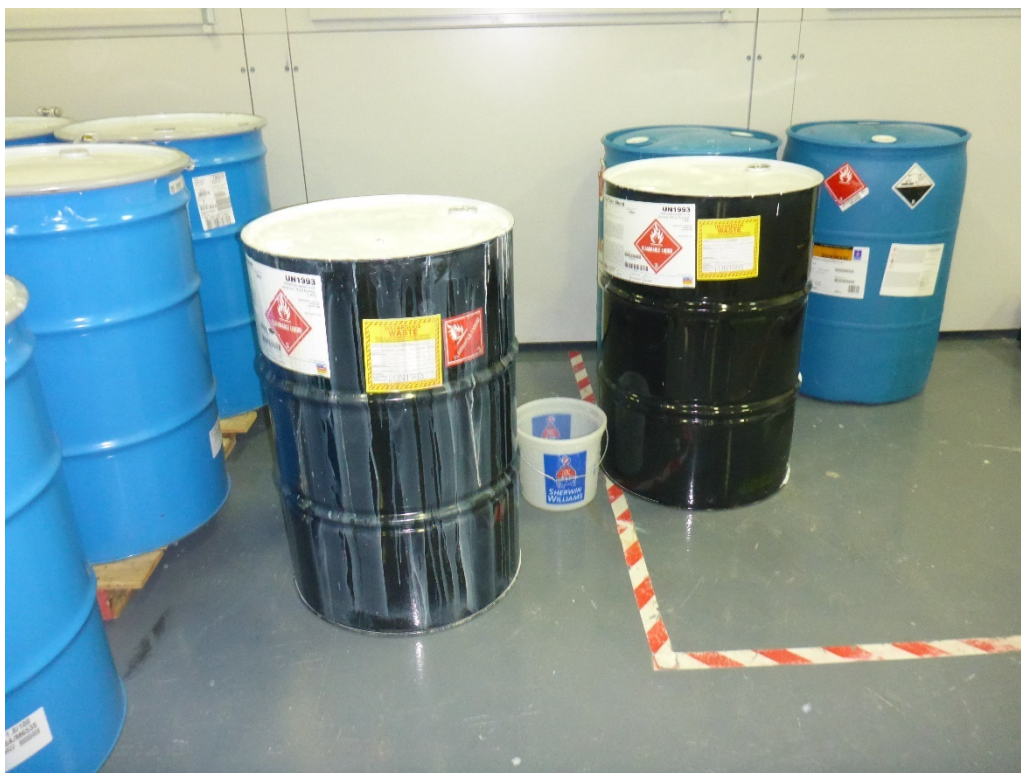
Photo 14: Two 55-gallon drums of hazardous waste observed with other 55-gallon drums at the end of the first solvent paint spray line. The drums were both labeled as D001 / F003 / F005 hazardous waste flammable liquid (acetone / toluene) and identified with a flammable liquid DOT hazard placard. One drum was dated 02/24/2021 and the other was dated 02/25/2021. Both drums also had product labels clearly visible for the original contents of the containers.
