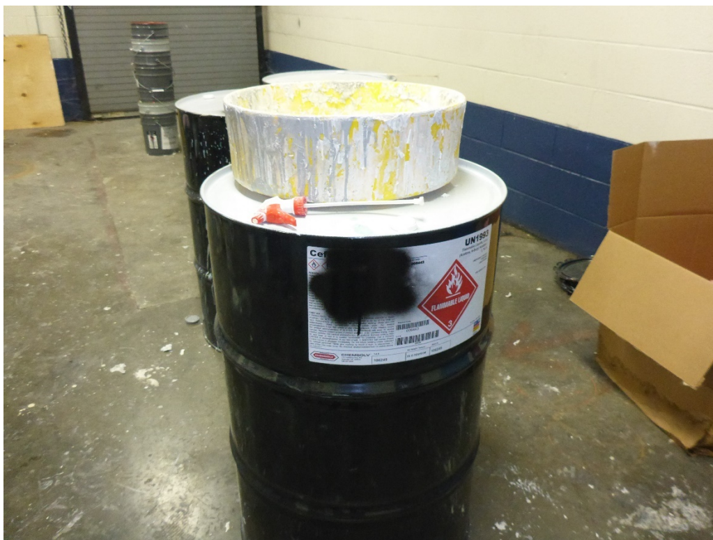
Photo 9: Another view of the 55-gallon drum observed near the wall opposite the solvent distillation unit in the Reclaim Room. According to facility personnel, this drum, which is equipped with an open funnel, is used to accumulate reclaimed Cefla Belt Cleaner solvent that is generated in the solvent distillation unit in this room.
