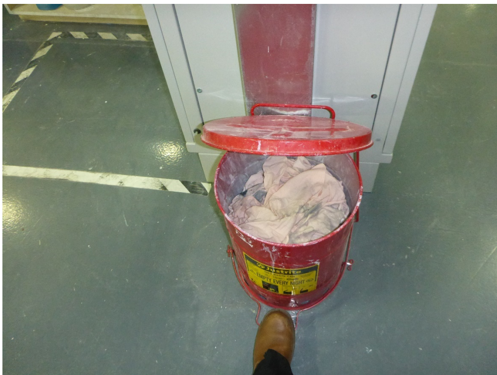
Photo 20: One 5-gallon step-open flammable can for accumulating excluded solvent contaminated disposable wipes at the second solvent paint spray line. The container is labeled as “oily waste” and “empty every night.” It is not labeled as excluded solvent contaminated wipes.
