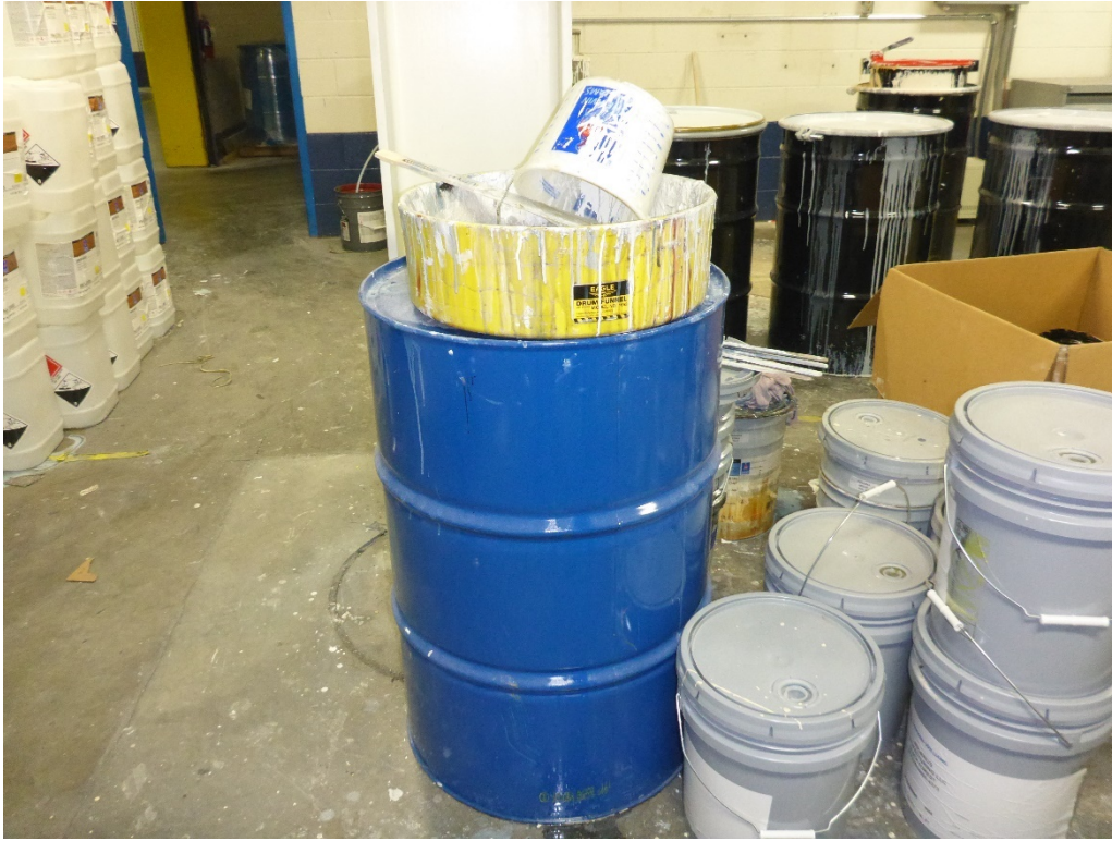
Photo 3: One 55-gallon drum observed near a post in the Reclaim Room. According to facility personnel, this drum, which is equipped with an open funnel, is used to accumulate waste UV paints that are brought into this room. Personnel stated that the standard operating procedure is to pour the contents of waste UV paint buckets into the designated 55-gallon accumulation drum located on portable secondary containment pallet in the UV Paint Coating Area along the wall just outside of the Paint Mixing Room shown in Photo #1. However, personnel working in this room maintain the accumulation drum shown in this photograph as a courtesy when employees mistakenly bring the 5-gallon containers of UV paint waste to this room.
