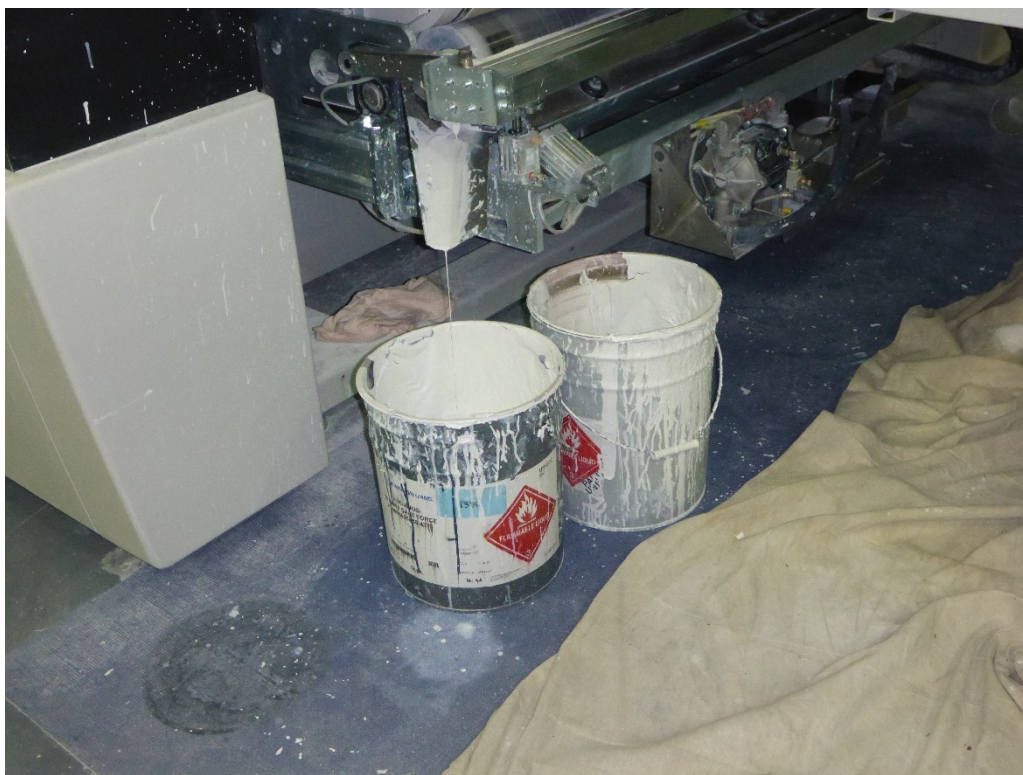
Photo 18: Two 5-gallon buckets staged at the second solvent paint spray line SAA. These buckets are used to accumulate D001 / F003 / F005 hazardous waste flammable liquid (toluene / acetone) that is generated as excess paint and overspray in this solvent paint spray line. Neither bucket is labeled with the words “hazardous waste.” Neither bucket is closed, but only one has waste being added into the container.
