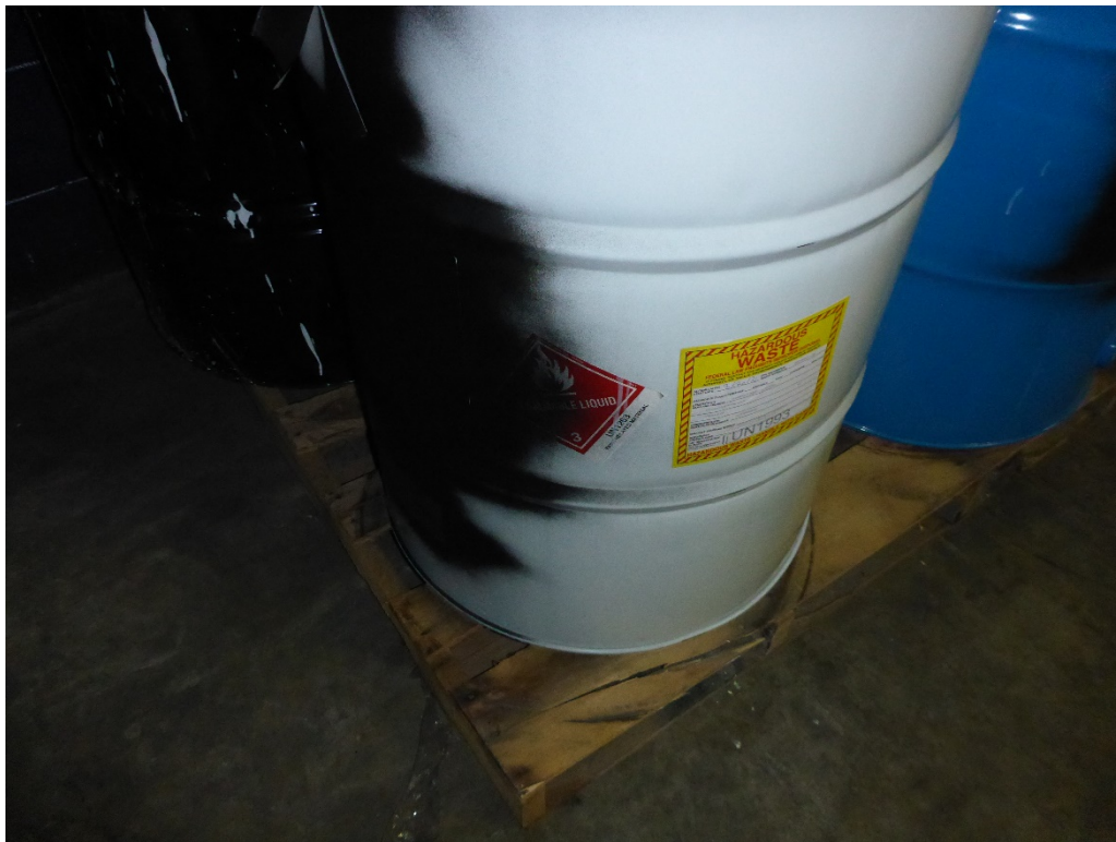
Photo 24: Partially covered flammable liquid DOT hazard placard on one drum in the hazardous waste CAA.
