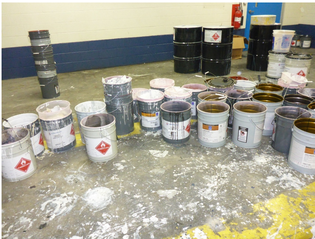
Photo 10: Several 5-gallon buckets with and without liners in the Reclaim Room. Buckets and liners appear to contain spent solvents, solvent paint waste and/or UV paint waste. The buckets are open and not labeled.
