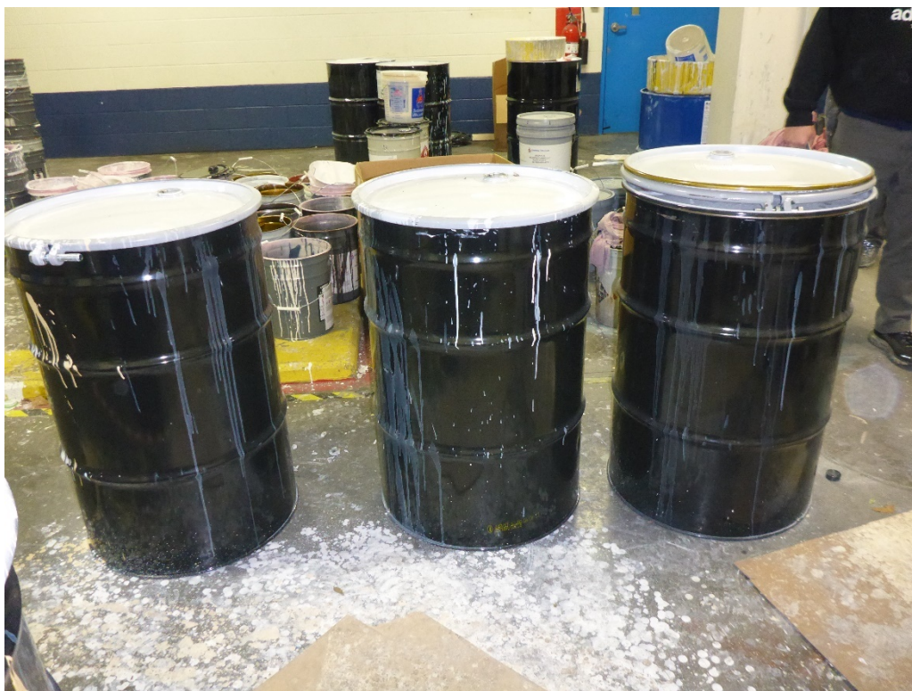
Photo 5: Three unlabeled 55-gallon drums observed near the solvent distillation unit in the Reclaim Room. Two of the drums are closed, but the drum on the right is open with no ring to secure the lid to the container. According to facility personnel, these drums contain spent Cefla Belt Cleaner solvent that is generated in the UV paint line. These solvents are staged here to be reclaimed in the solvent distillation unit, and the reclaimed solvent will be reused in the UV paint line.
