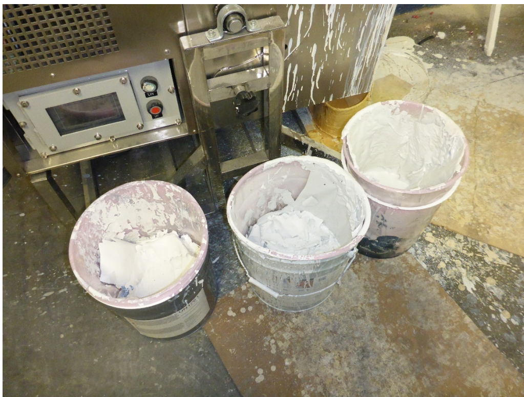
Photo 7: Three 5-gallon buckets in front of the solvent distillation machine that contain an unknown material and may be used to load spent solvents into the machine and/or unload solvent sludge from the machine.
