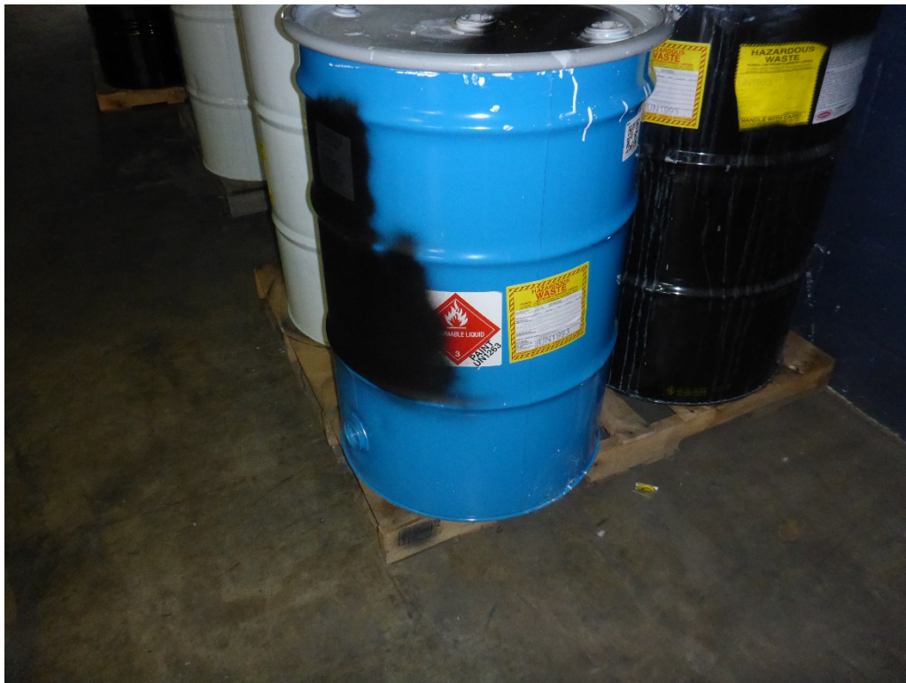
Photo 23: Partially covered flammable liquid DOT hazard placard on one drum in the hazardous waste CAA.
