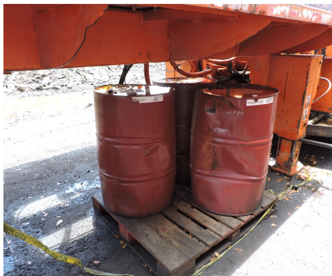
Picture 34 - DCN RECYCLING, CORP. - As observed during the EPA Inspection, all drums containing leaking fluids from crushing operations are managed as used oil and disposed of with Ruben Martinez Used Oil Collection Services. No hazardous waste characterization is performed on the leaking fluids from the crushing operations on routine basis.
