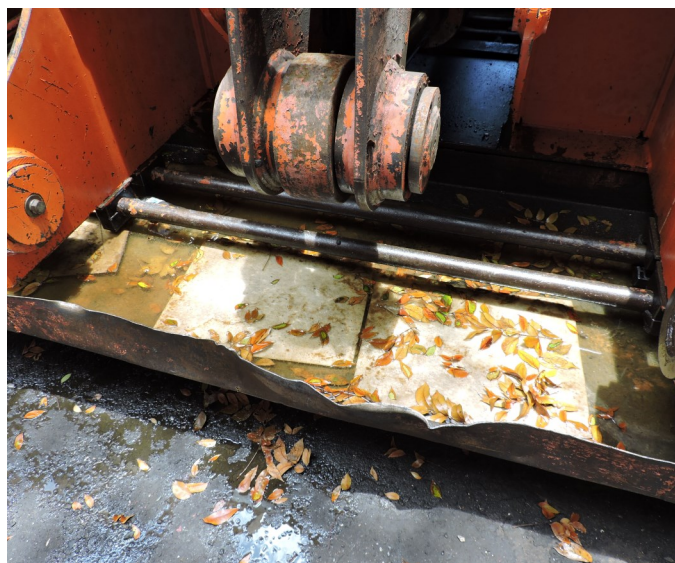
Picture 6 - DCN RECYCLING, CORP. - As observed during EPA Inspection, all mixed fluids generated from crushing and compacting operations are trapped into a metal tray-typed and collected with absorbent materials.
