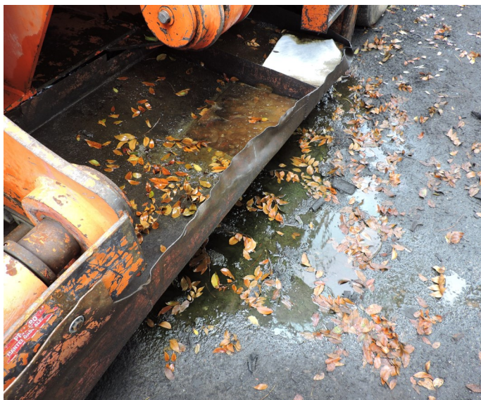
Picture 33 - DCN RECYCLING, CORP. - As stated by EPA, junked cars contained components that were potential hazardous materials such a gasoline residue in the gas tank and any fluid leaks generated during crushing is collected in the steel tray and/or 55-gallon drums.
