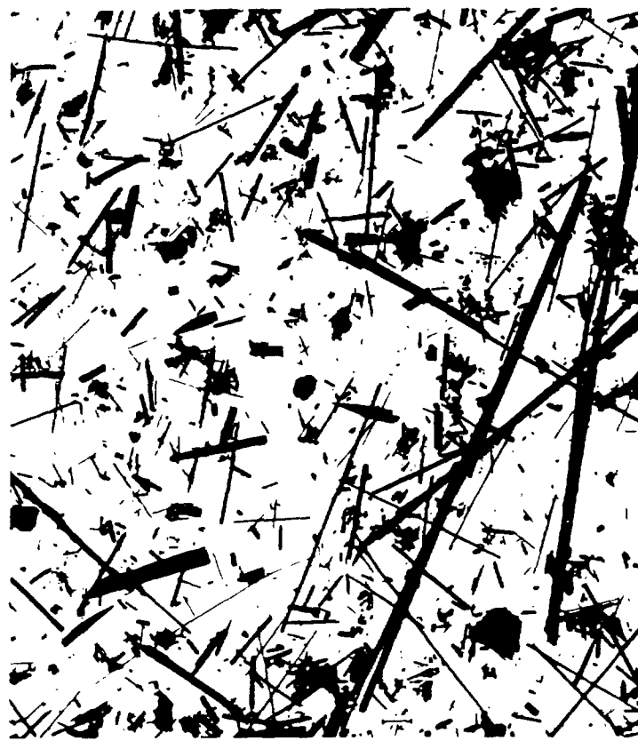
FIG 2—Electron mi- crograph of crocidolite. X8000. Reduced ap- proximately 33% in reproduction.
