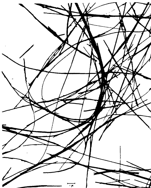
FIG. 1—Electron micrograph of Jeffrey chrysotile. X8000. Reduced approximately 33% in reproduction.
