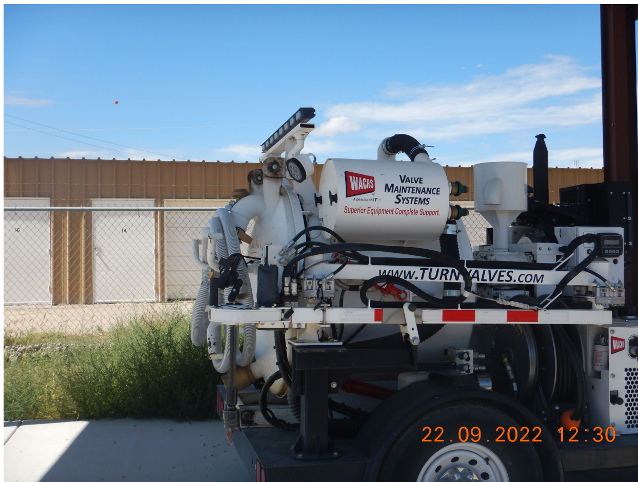
View of Operation and Maintenance (O&M) equipment (specifically valve maintenance) used by the City of Rio Rancho (DSCN2338) Photographed by D. Esparza
