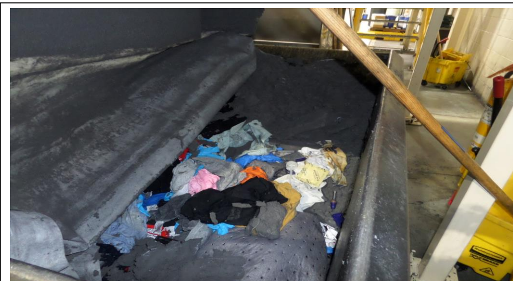
Hyundai. Engine Building 1. Inspectors observed a container accumulating metal solids, grease and oily grime from filtering coolant used in the engine machining operation. The filtered metal solids are accumulated in a 0.5 cubic yard container. Photograph 21 taken July 27, 2021 at 11:09 a.m.
