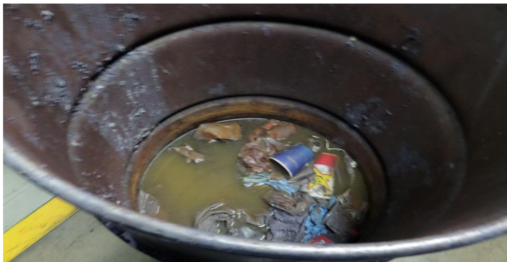
Hyundai. Contractor Paint Area. Inspectors observed seven 55-gallon containers on pallets along the wall accumulating unknown solid waste. One open container was accumulating waste liquid and trash (paper towels and cups). Inspectors observed four containers were accumulating various amounts solid waste. Photograph 4 taken July 26, 2021 at 3:03 p.m.
