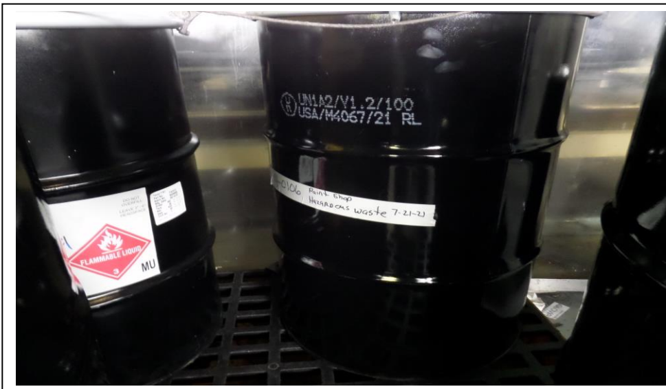
Hyundai. Top-Coat 90-Day Area. The inspectors observed four 55-gallon containers accumulating hazardous waste on a poly pallet. One container was not marked/labeled with a hazard indication and not marked with waste codes. The facility marked the container with an ignitability indication and with the waste codes D001, F003. Photograph 16 taken July 26, 2021 at 3:59 p.m.
