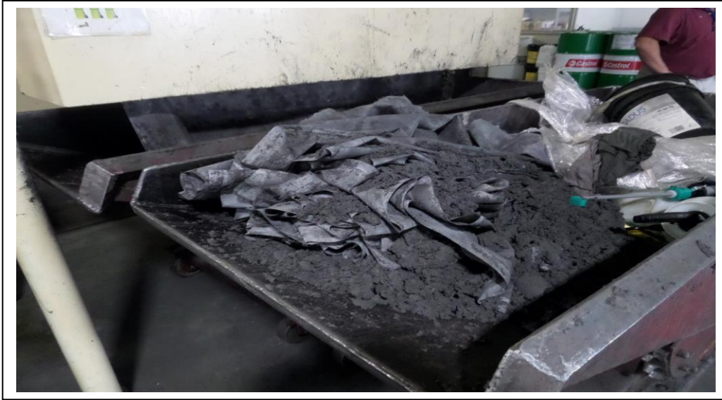
Hyundai. Engine Building 2. Inspectors observed a container accumulating metal solids, grease and oily grime from filtering coolant used in the engine machining operation. The filtered metal solids are accumulated in a 0.5 cubic yard container. Photograph 23 taken July 27, 2021 at 11:28 a.m.
