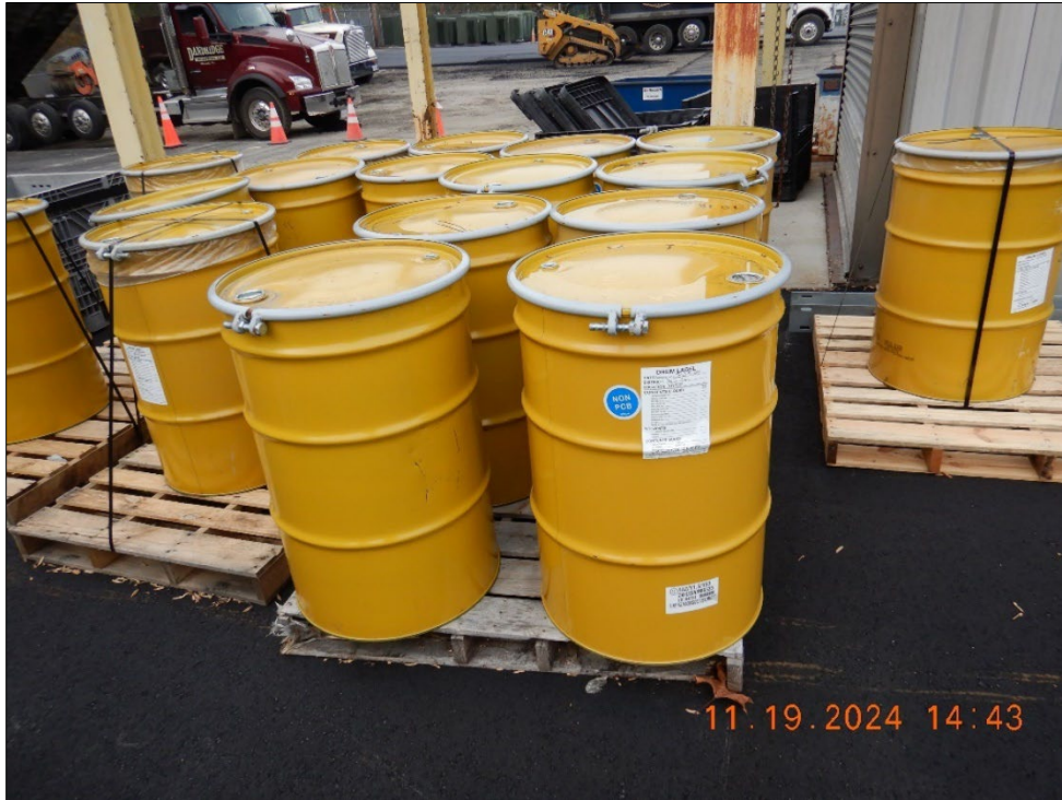
Photograph 11. DSCN0608.JPG View of drums of waste lamps that were sealed and labeled.
