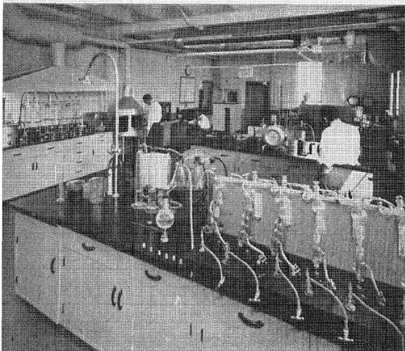
The distillation test is one of many standard methods of the American Society for Testing Materials used by field laboratories.
