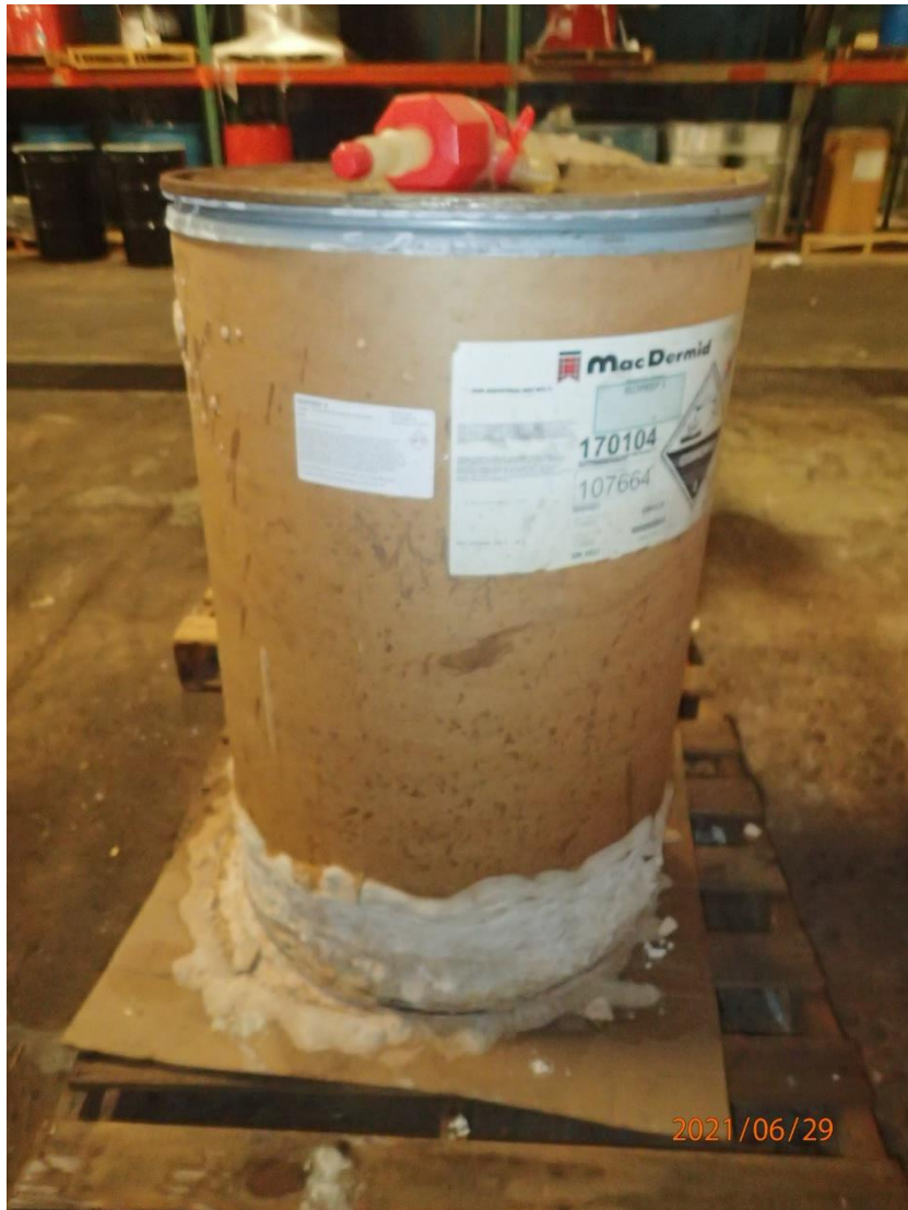
Photo 14: One (1) 55-gallon fiber drum of Isoprep 3, closed but appeared to show evidence of leaking around the bottom of the drum. The drum had a corrosive placard to indicate its hazard contents and a product expiration date of 11-20-19.
