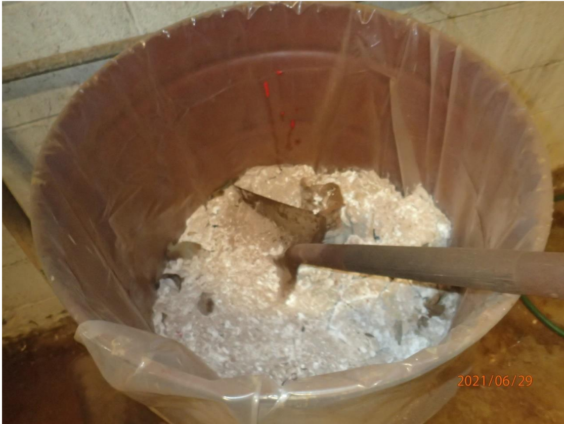
Photo 4: 55-gallon drum with what appeared to be floor sweepings, was observed open and not labeled. Facility personnel were unsure if the material was hazardous or non-hazardous waste when asked.
