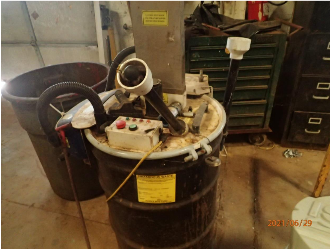
Photo 2: 55-gallon SAA drum with a bulb crusher on top, labeled “Hazardous Waste – Crushed Lamps”, closed, but did not indicate the hazard of the contents.
