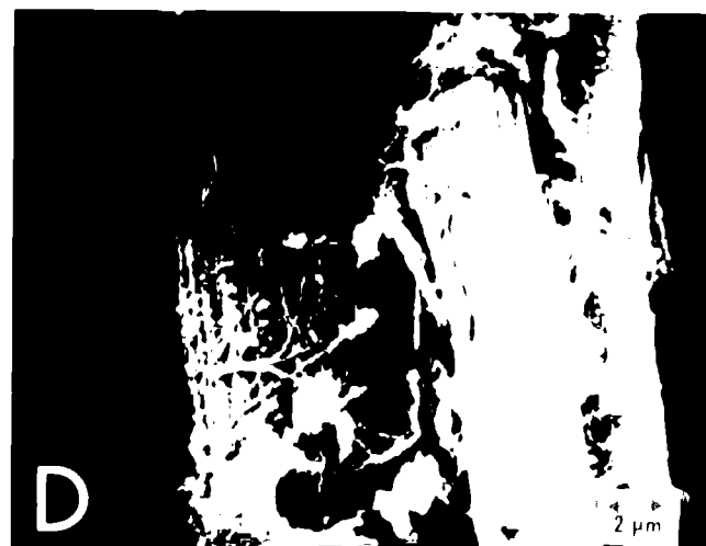
Fig. 3. Photomicrographs of debris from laboratory bench top and laboratory wall. A. Full-field of bench top debris (initial magnification, \times 50 ). B. Full-field of wall debris (initial magnification, \times 50 ). C. Linear component of bench top debris (initial magnification, \times 5,000 ). D. Bundle of linear components of wall debris (initial magnification, \times 5,000 ).
