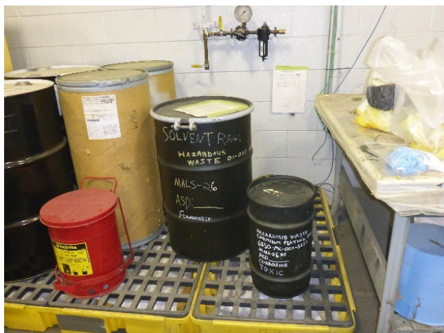
Photo 14: One 35-gallon container for accumulating hazardous waste rags generated from solvent cleaning activities and one 5-gallon container for accumulating hazardous waste rags generated in the cadmium plating process in the MALS 26 Air Frames Metals Shop SAA.
