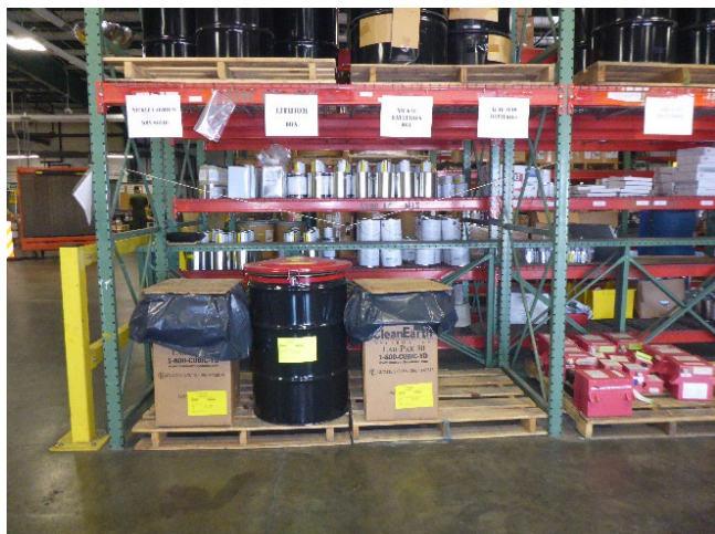
Photo 1: Bay A1 for consolidating and storing nickel-cadmium dry-solid batteries, lithium-ion batteries, nickel batteries dry, and lead acid batteries in the CAA.
