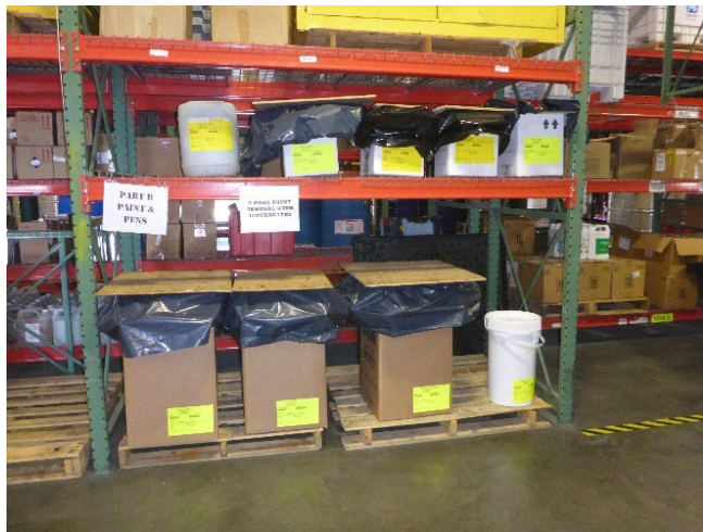
Photo 5: Bay A5 for consolidating and storing part B paint and pens and two-part aerosol with isocyanates in the CAA.
