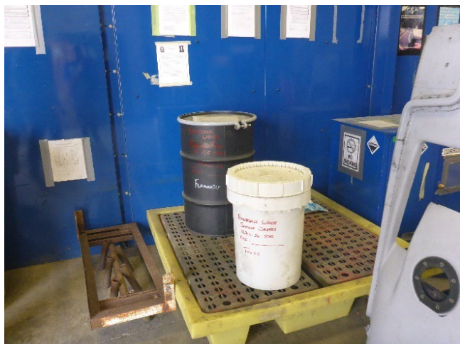
Photo 16: One 30-gallon container for accumulating hazardous waste solvent rags and one 20-gallon container for accumulating hazardous waste sanding debris in the MALS 26 Air Frames Composite Shop SAA.
