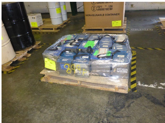
Photo 13: Pallet of lead-acid batteries ready for shipment in the CAA. Batteries shrink-wrapped together. Shrink-wrapped was labeled universal waste batteries, but individual batteries were not labeled.
