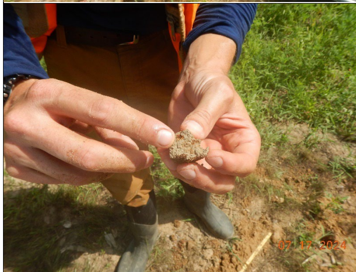
Paul Goodwin Date: 17 July 2024 Photo ID: DSCN5539.JPG Photo taken by: Laura Mathew Notes: Close up view redoximorphic features present in the native hydric soil located at >21" below ground surface.
