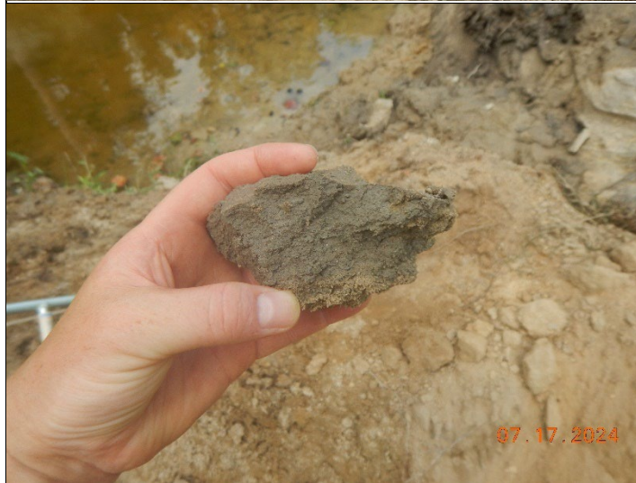
Paul Goodwin Date: 17 July 2024 Photo ID: DSCN5518.JPG Photo taken by: Laura Mathew Notes: Close up view of fill material comprising the berm. Note the reduced matrix and redoximorphic features.
