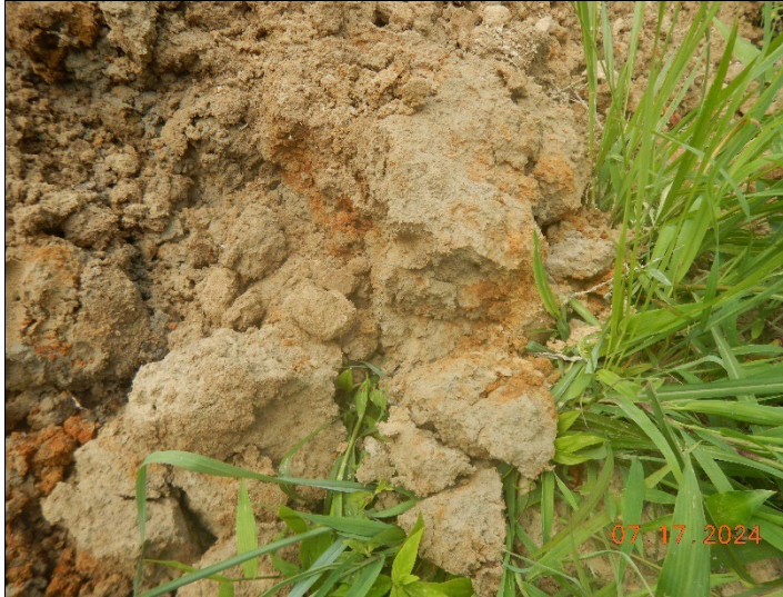
Paul Goodwin Date: 17 July 2024 Photo ID: DSCN5522.JPG Photo taken by: Laura Mathew Notes: View of depleted matrix and redoximorphic features in the unconsolidated material comprising the berm.
