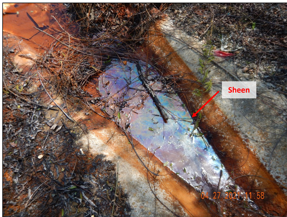
DSCN2363. Another view of surface sheen in the dry-weather flow to Outfall 911.
