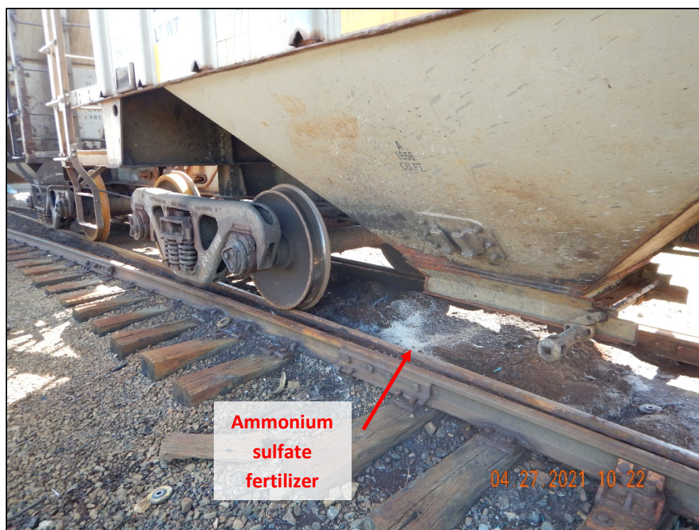
DSCN2319. View, facing southeast, of ammonium sulfate fertilizer on the ground beneath a rail car hopper.
