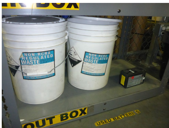
Photo 6: Two 5-gallon buckets for accumulating spent batteries, and one spent lead-acid battery observed on a shelf inside the battery cage. One bucket was labeled for spent lithium batteries, one was labeled for spent alkaline batteries, and the lead-acid battery was dated June 26, 2023.
