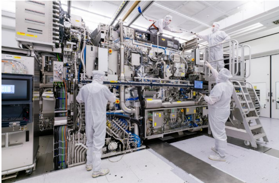
Figure 10-1 ASML Latest Extreme Ultraviolet Photolithography Exposure Tool. 79
