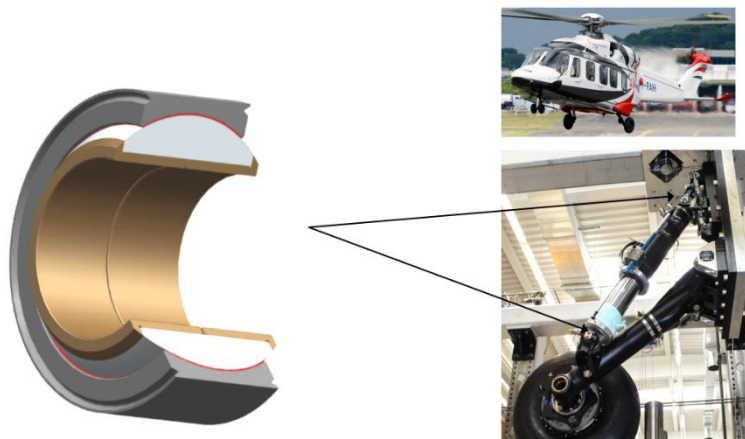
figure 8: Liner bearing in the landing gear of a helicopter
