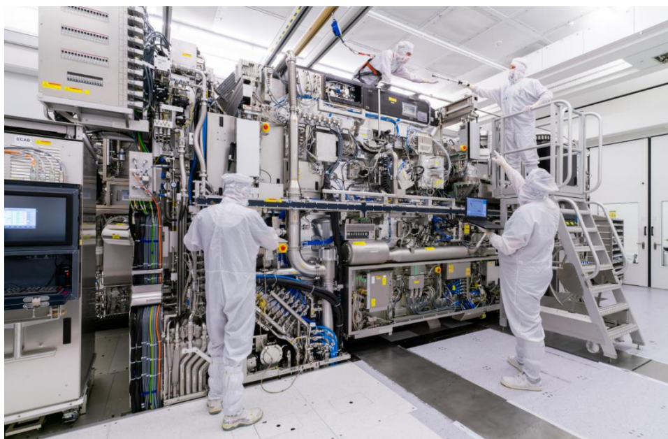
Figure 3: Dutch firm ASML’s latest EUV photolithography exposure tool (Source: ASML).
