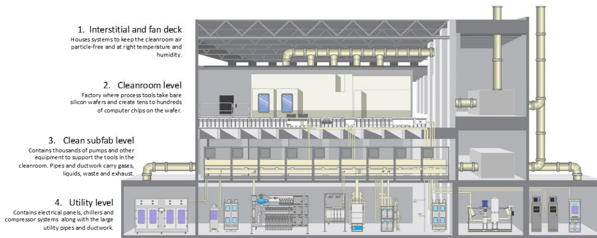
Figure 17: Example semiconductor manufacturing facility layout (CPS and Exyte Group Company 2019).
