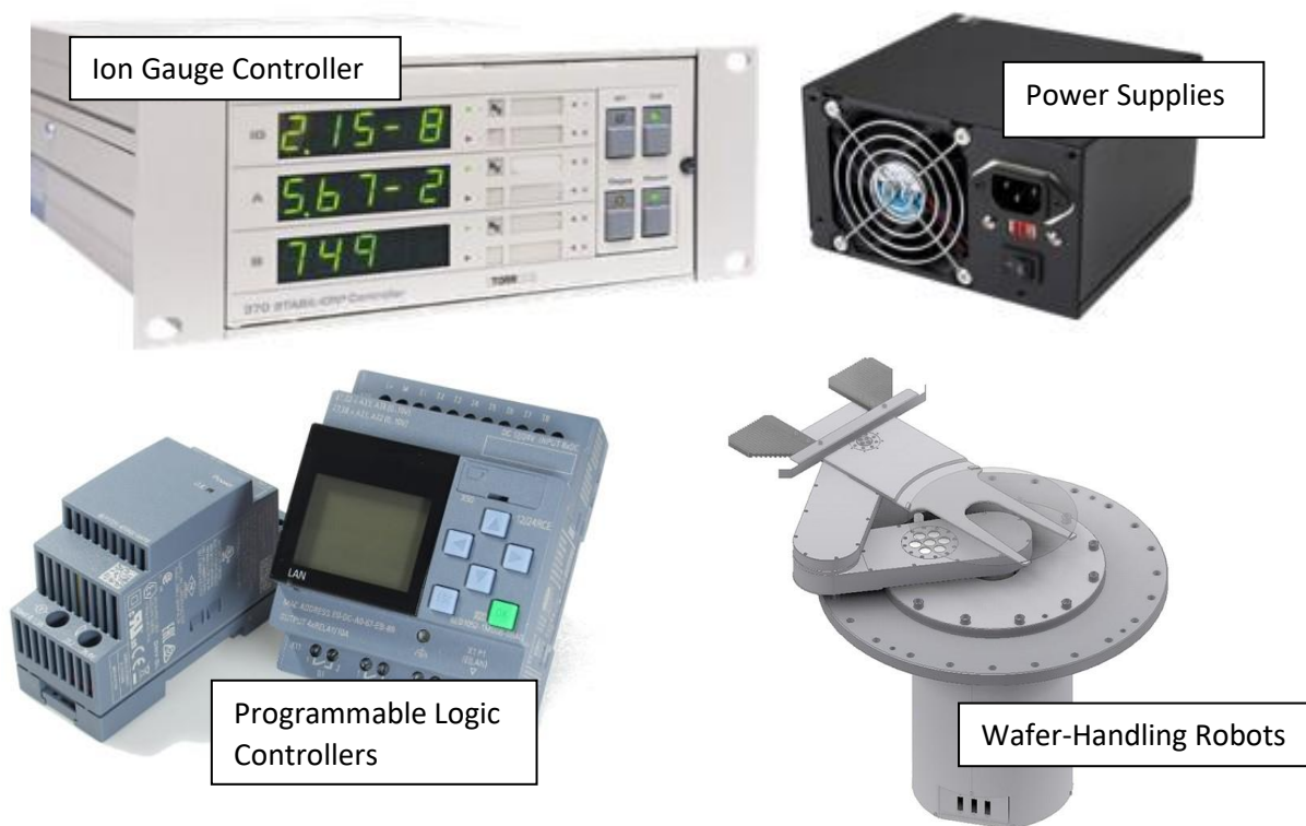
Figure 7: Examples of complex assembly components that could contain PFAS.
