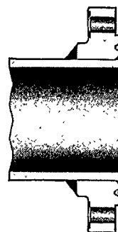
Ring Joint on Slip-On Welding Flange
