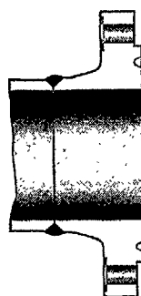
Ring Joint on Welding Neck Flange
