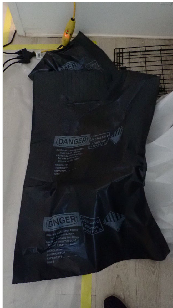
Figure 5: Black asbestos waste bag.
