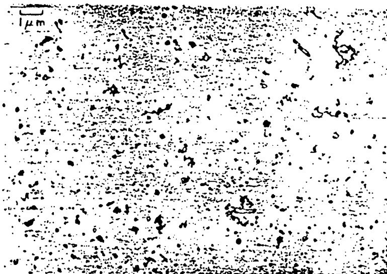
FIG. 1. Particulate matter filtered from London air.
