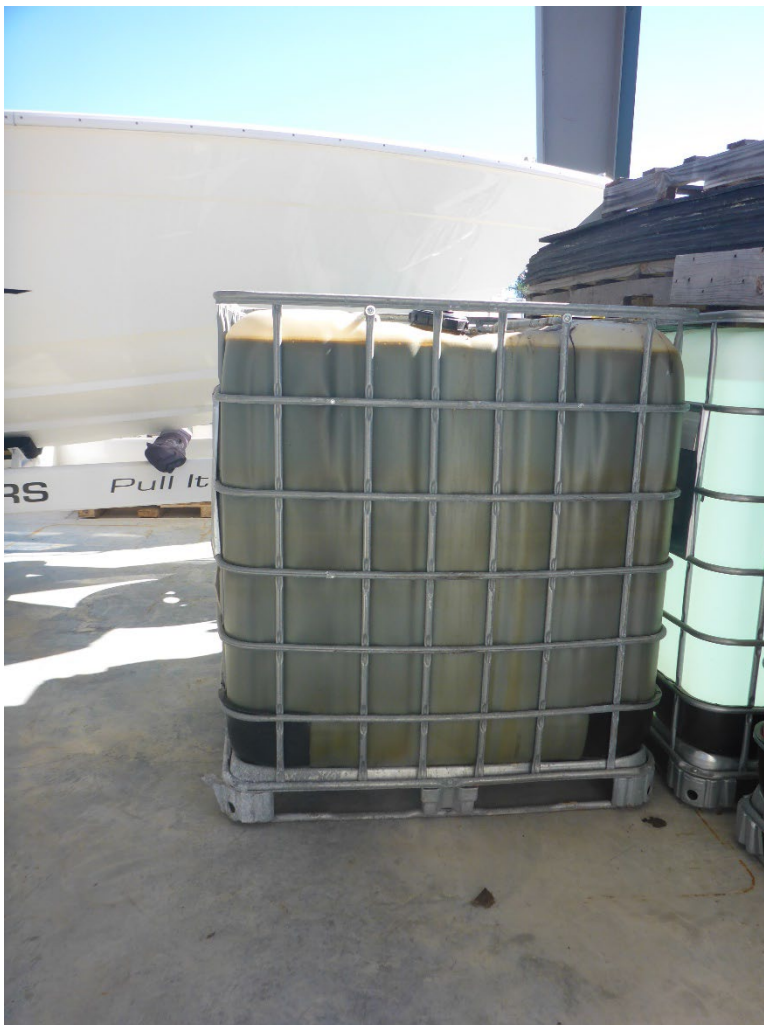
Photo 6: One 330-gallon tote of hazardous waste staged beneath a roof on a concrete pad just outside of the blending facility area. According to facility personnel, this is the first full tote of laboratory hazardous waste that has been generated at the facility, and it was moved to this area approximately one week prior to the inspection. The container was not labeled with the words “hazardous waste,” it was not marked to indicate the hazards of its contents, and it was not marked with an accumulation start date.
