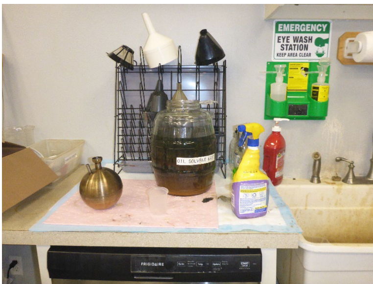
Photo 1: One 2-gallon glass container in Main Laboratory SAA. The container was not labeled as hazardous waste or identified with an indication of the hazards of its contents.
