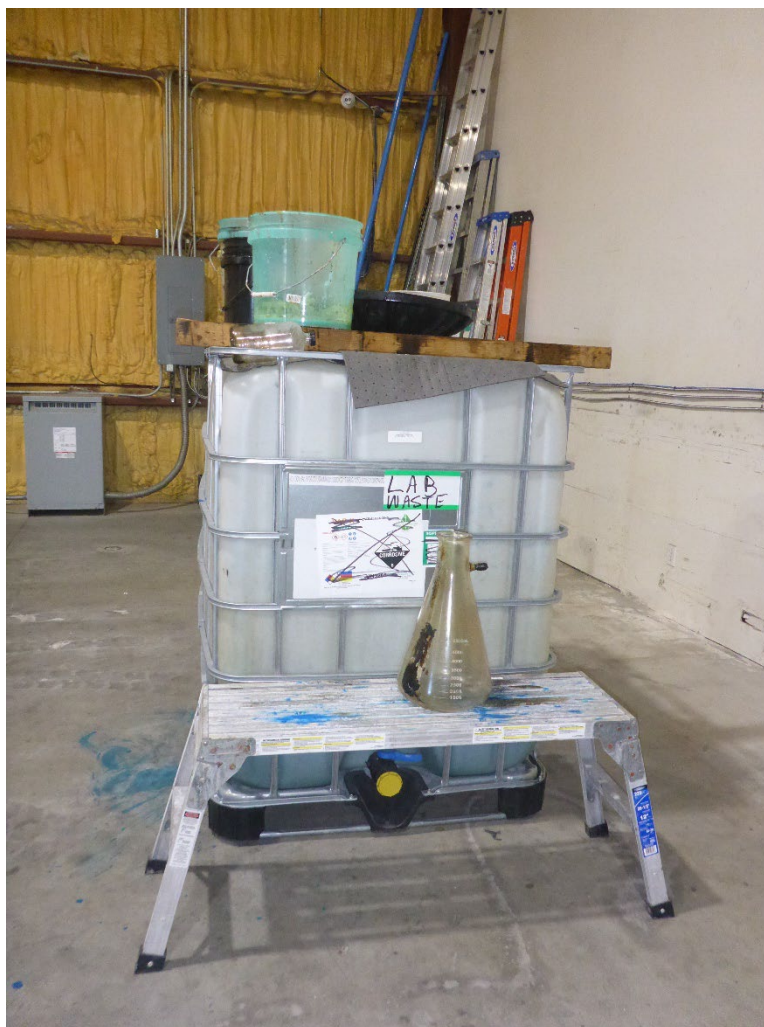
Photo 3: One 300-gallon tote of hazardous waste in a CAA just outside of the Main Laboratory. The container was labeled "lab waste." The container was not labeled with the words "hazardous waste;" it was not marked with an indication of the hazards of its contents; and it was not marked with an accumulation start date. The container was equipped with a funnel sitting on top of the tote, but the funnel and the container were both open.
