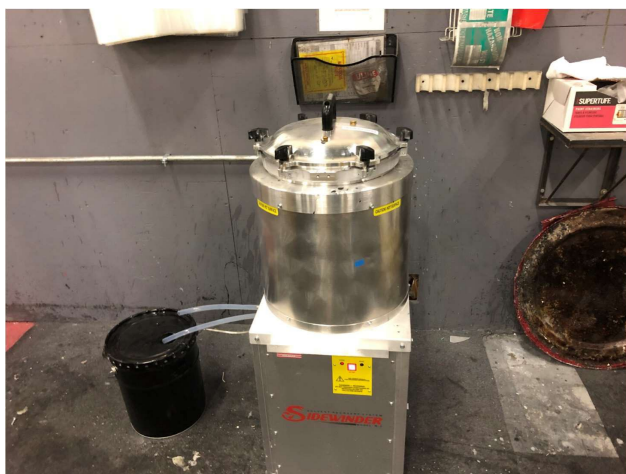
Photo 8: Solvent Recovery System 2.
