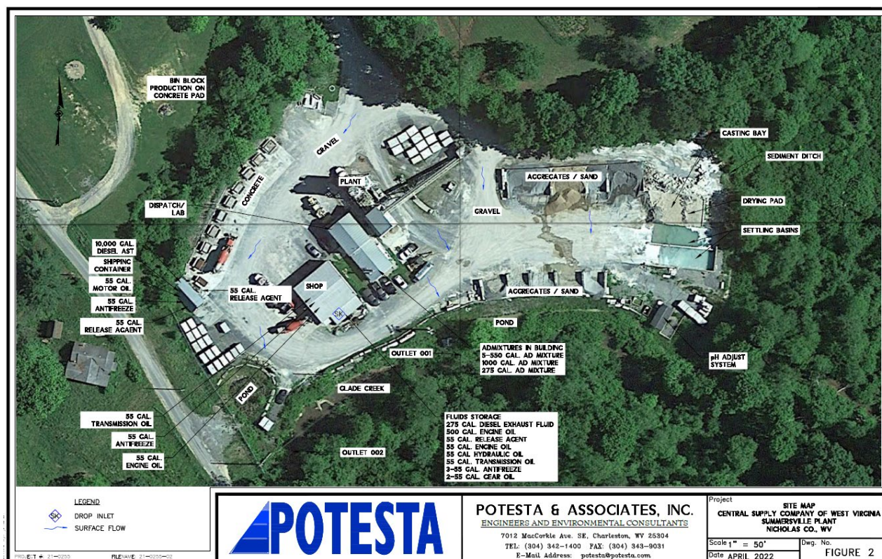
Figure 1. SWPPP Site Drainage Map
